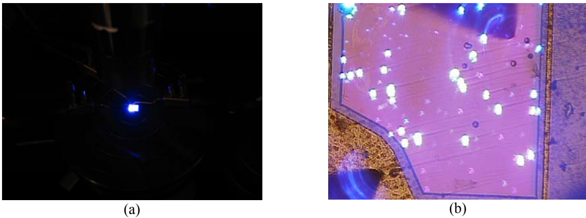
Figure 32: (a) Bird's eye view of light emission and (b) picture of light output (at low current level) from fabricated LED devices grown on a (11-20) a -plane GaN bulk substrate.
