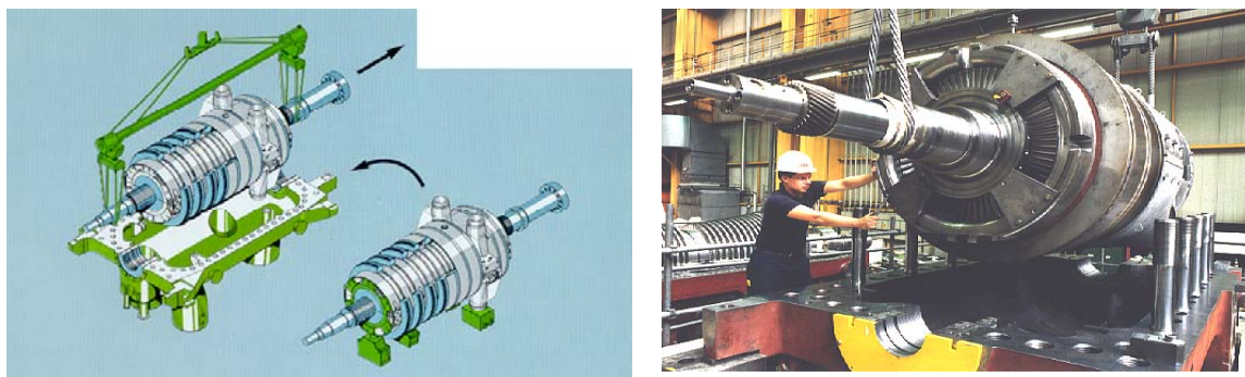
Figure 5-2: HP Inner Block Retrofit Illustrating "Drop In Solution"
