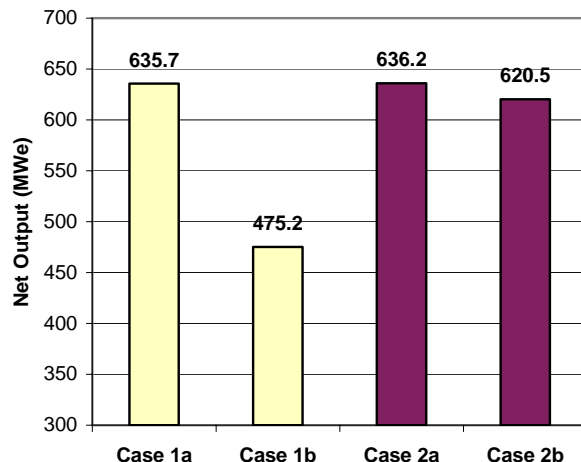
Figure 3-5: Net Plant Electrical Output Comparison
