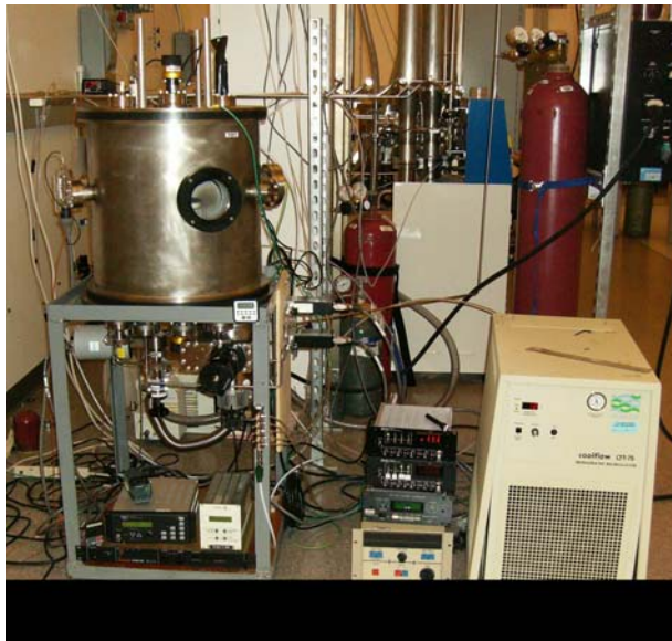
Fig. 9 CVD system being assembled at Solasta for development of conformal TCC. The initial target material will be Al-doped ZnO.
