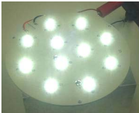
Figure 15: Experimental high flux lamp module consisting of an array of individual emitters on a metal core circuit board.
