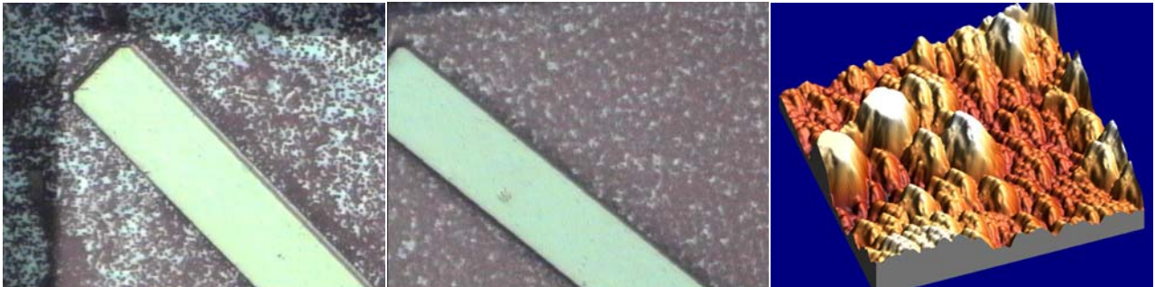
Figure 6: (a) Example of optical micrograph of surface of LED subject to one particular roughening etch process. (b) Same except longer etch time. (c) Atomic force micrograph of 20 x 20 \mu\text{m}^2 portion of surface in (b).
