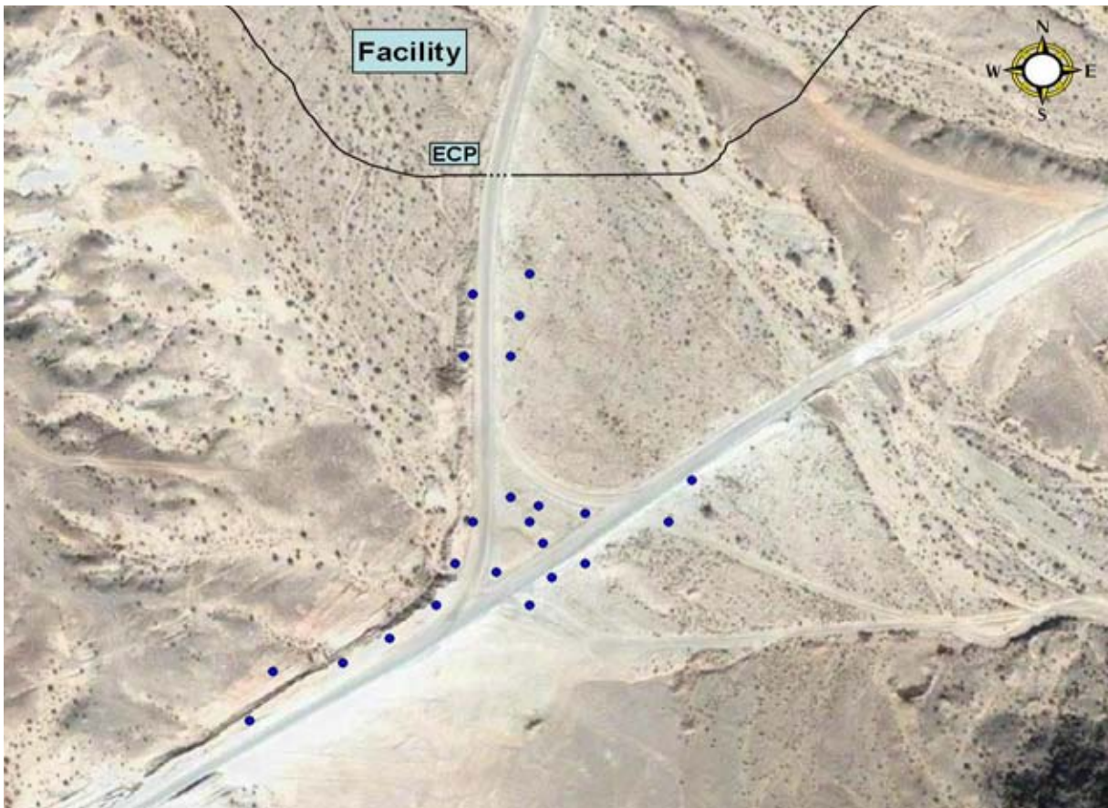
Figure 8 Vehicle tracking scenario map. Blue dots are seismic/acoustic sensor nodes.
