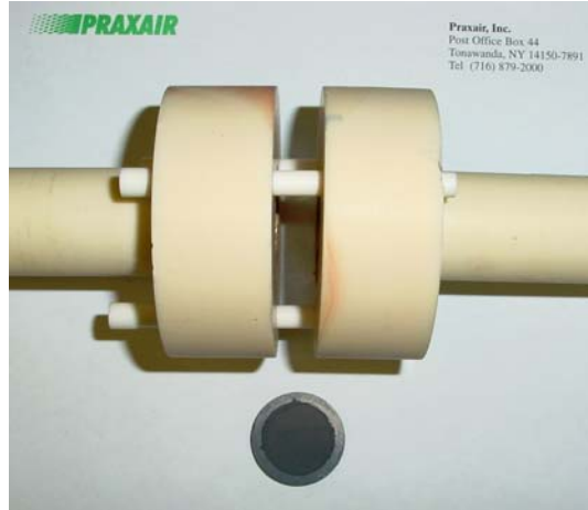
Figure 14, a) Experimental setup for disc reactor, b) Close-up of the actual disc reactor in which the OTM disc gets clamped between two tubes.
