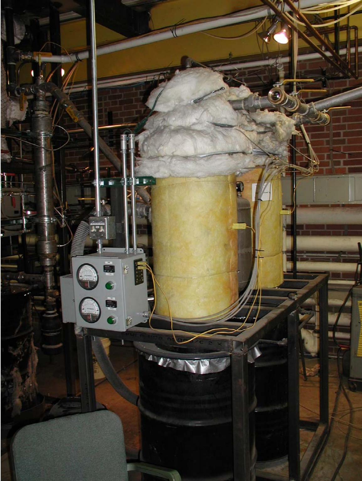
Figure 13: Photograph of two single-bag baghouses removing ash for the UND Chemical Engineering 19 kW research combustor
