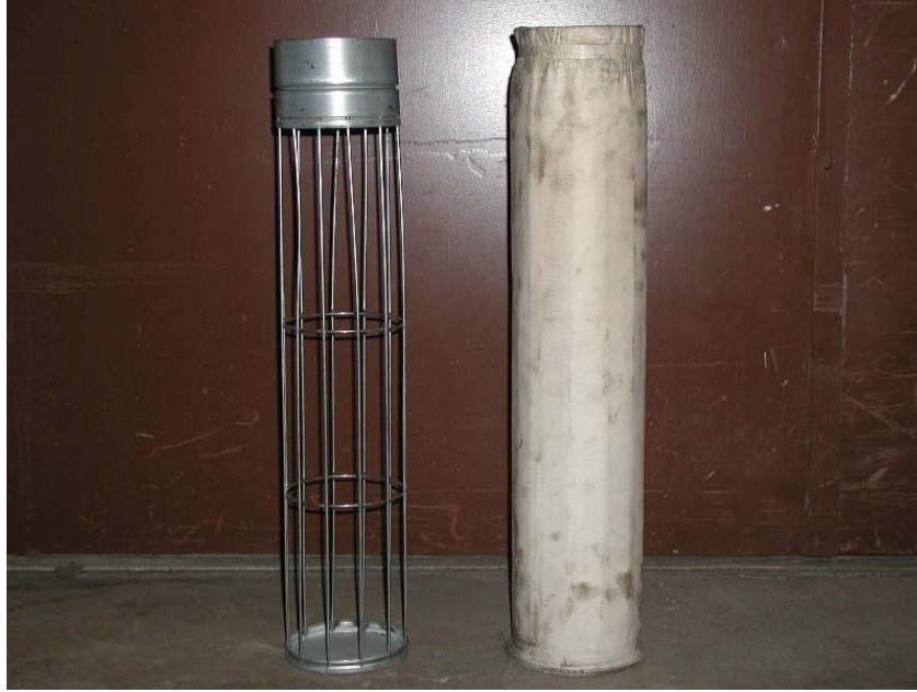
Figure 14: Photograph of baghouse filter cage and baghouse filter used in baghouses for UND Chemical Engineering 19 kW research combustor
