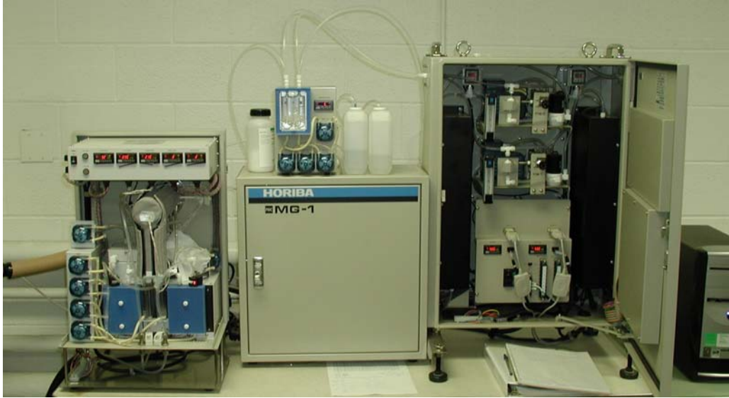
Figure 4: Photograph of the complete Horiba unit. The DM-6B analyzer is on the right, the MS-D1 conditioning unit is on the left, the MG-1 mercury generator is in the center, and the SO 2 scrubber is located on top of the MG-1
