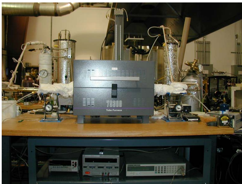
Figure 37. Picture of the modified test rig, capable of operating in the SOFC, SOEC, and SOFEC modes
