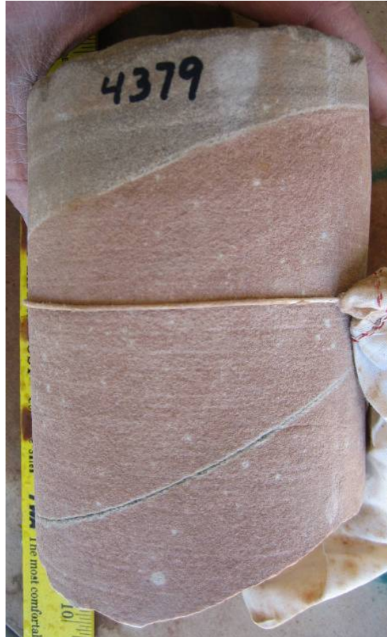
Figure 2.24 Steeply inclined, regular cross bedding of well-sorted, fine-grained sandstone, representing the deposits of an eolian dune environment, as seen in core. One of the bedding planes is highlighted by gray discoloration, suggesting enhanced permeability along this plane. The overlying gray bedding is nearly horizontal and on laps the inclined dune foresets.
