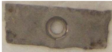
Figure 27. Photographs of Nb-1Zr alloy of the after exposure to molten salt at 850C for 500 hours, showing sever corrosion and embrittlement.
