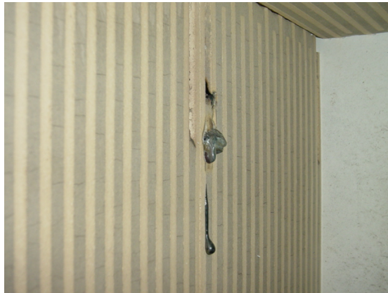
Figure 13. Some heating elements in the high temperature furnace failed and had to be replaced and the furnace was subsequently operated satisfactorily.
