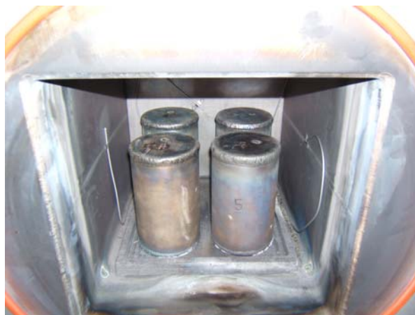
Figure 9. The crucibles to be tested were placed in the argon atmosphere furnace, which was heated to 850°C.
