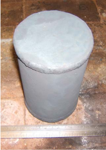
Figure 17. Photograph of the oxidized stainless steel capsule after exposure at 1000°C for 500 hours, in air.
