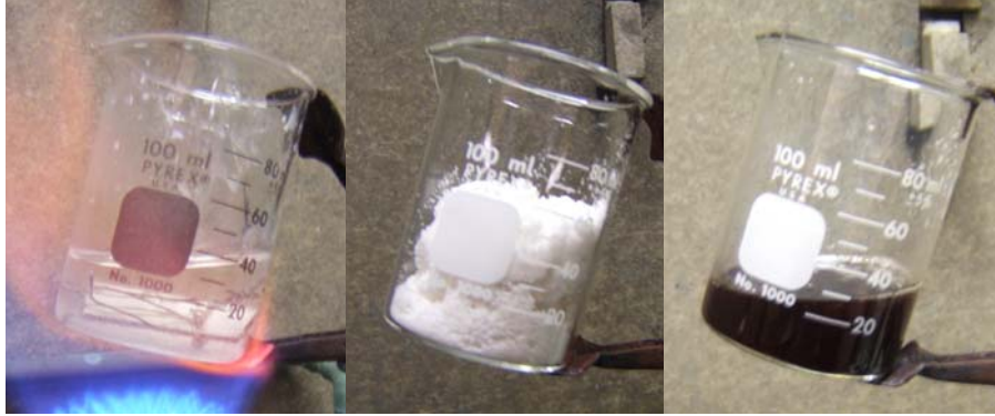
Figure 12. Removal of solidified salt from test samples using 1 M \text{Al}(\text{NO}_3)_3 .
