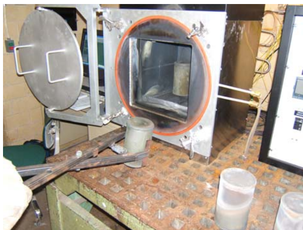
Figure 10. The corrosion capsules were inverted at 500°C after testing at 850°C for 500 hours.
