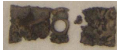
Figure 27. Photographs of Nb-1Zr alloy of the after exposure to molten salt at 850C for 500 hours, showing sever corrosion and embrittlement.
