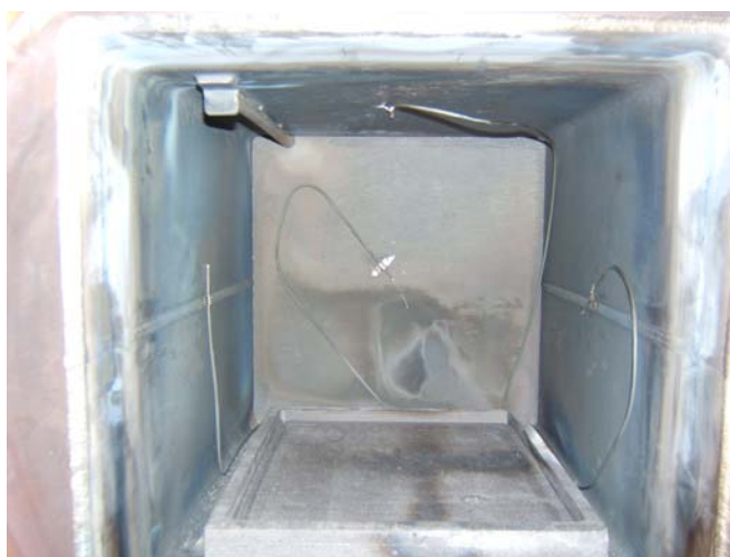
Figure 15. Photograph of the argon atmosphere furnace showing thermocouples and graphite spill tray.
