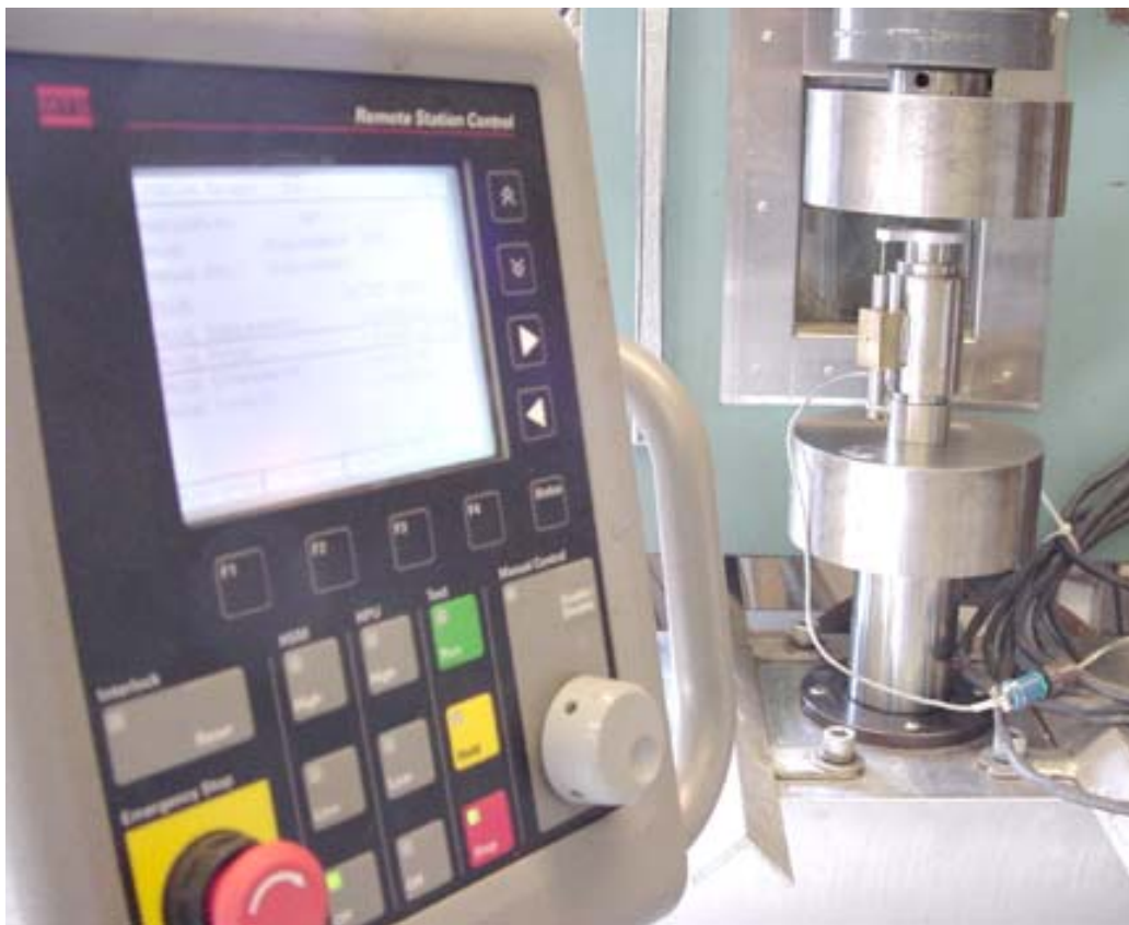
Figure 16. Uniaxial strain compression test set-up controlled by a servo-controlled system.
