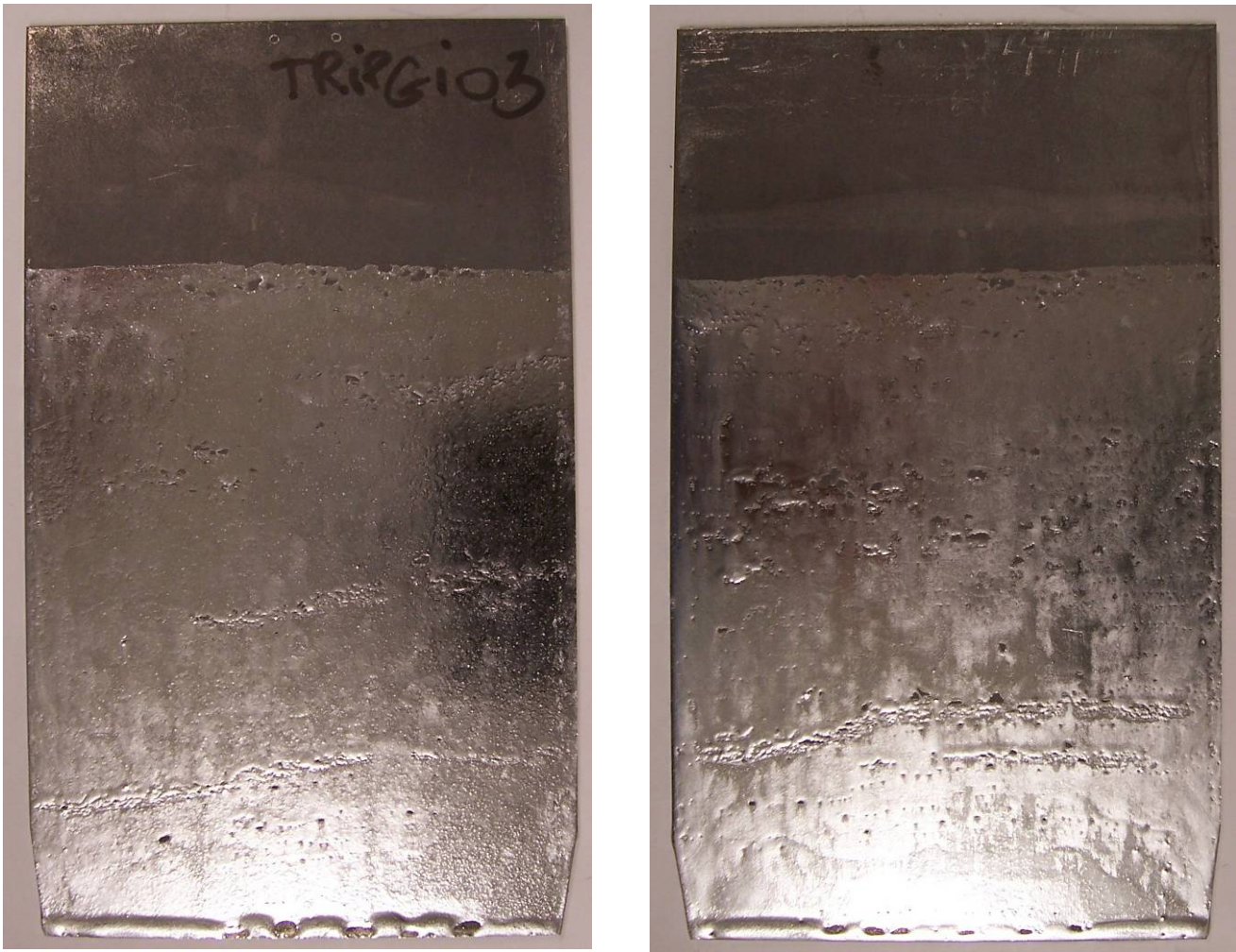
Fig. 71 – Example of a TRIP coupon galvanized according to schedule TRIP-GI03 (see Table 16).
