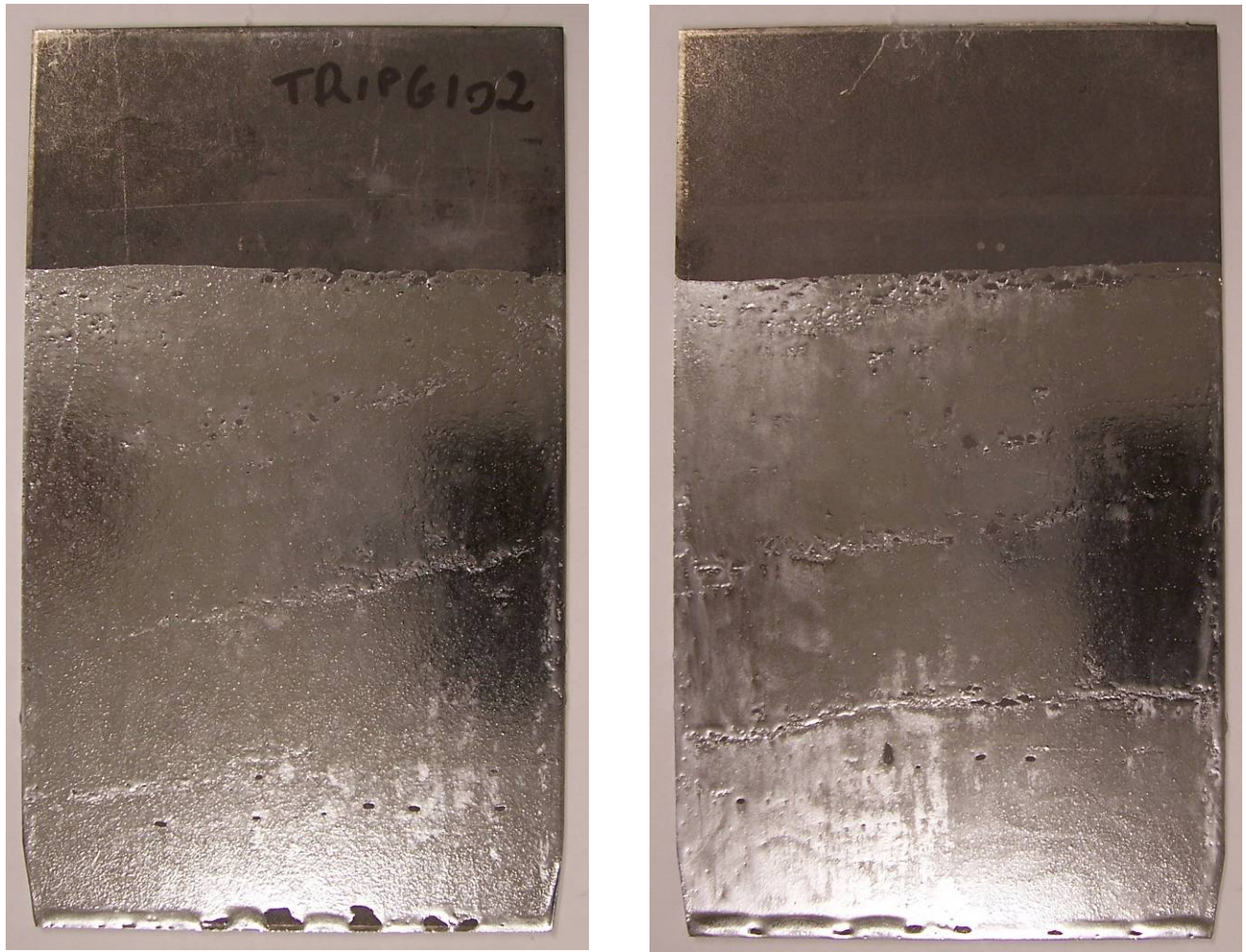
Fig. 70 – Example of a TRIP coupon galvanized according to schedule TRIP-GI02 (see Table 16)
