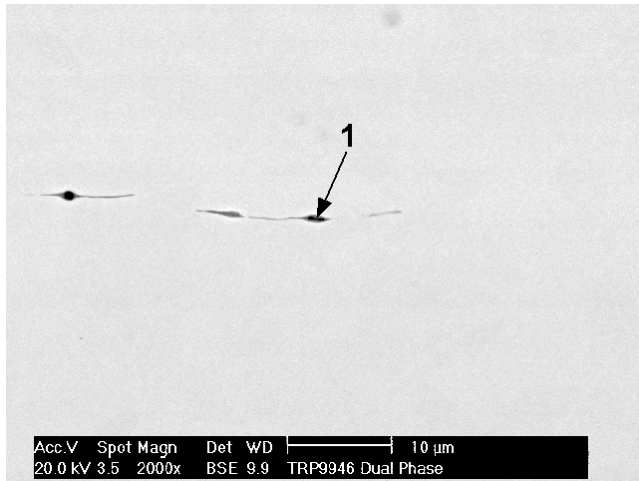
(a) BSE micrograph of an elongated MnS inclusion (spot 1).
