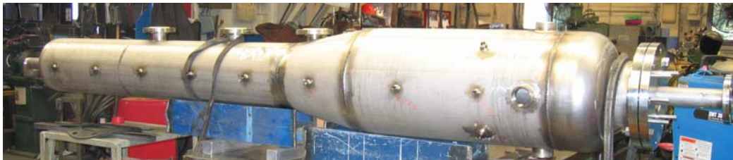
Figure 5.10 Tube bundle condenser secondary pool tank
