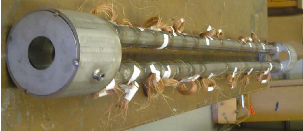
Figure 5.7 Picture of the condenser tube bundle with thermocouples mounted on the tubes.
