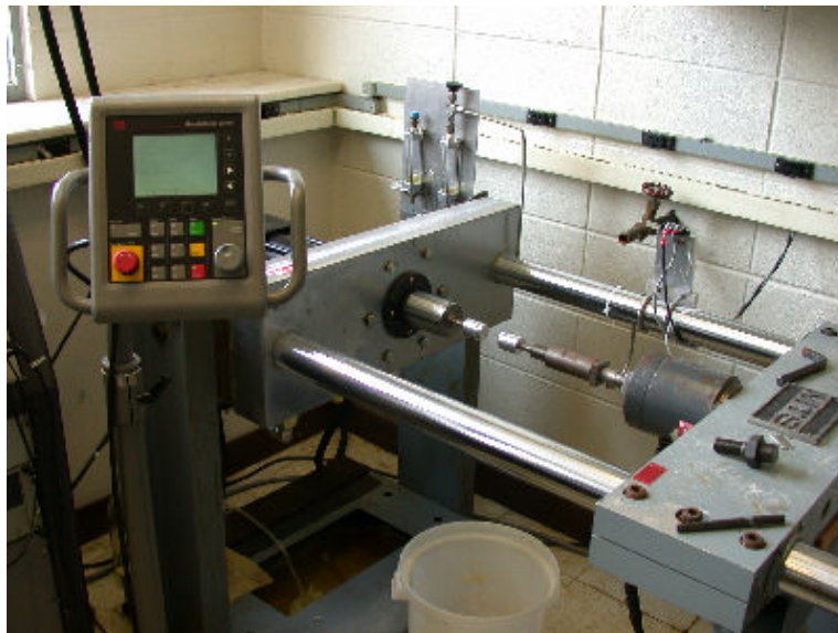
Figure 3.9: Tensile butt joint fatigue setup.
