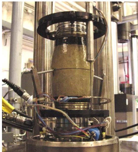
Figure 5. Instrumented Big Hill salt specimen exposed after triaxial compression testing. Shown are two axial LVDT's and a Schuler gage mounted on the specimen to measure axial and the lateral displacements, respectively.
