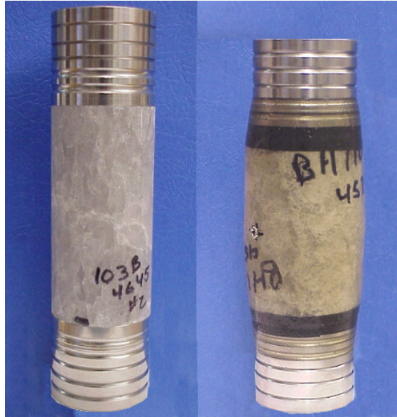
Figure 4. Big Hill salt specimens (left-before testing without coating; right-after testing with polyurethane coating).
