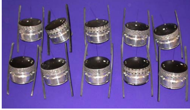
Figure 18. Hopping landmine robots used in self-healing minefield tests.
