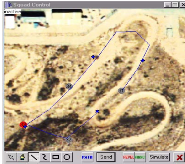
Figure 15. Four robot vehicles are shown guarding a perimeter denoted by the blue line segments. When an intrusion detection sensor denoted by the numbered circles alarms, one robot vehicle attends to the alarm (vehicle near sensor 33) while the others spread apart along the perimeter so that each vehicle is midway between its neighbors.
