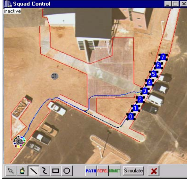
Figure 23. Robot path planner drives vehicles towards ellipse while staying away from obstacles, denoted by red line, and the other vehicles.
