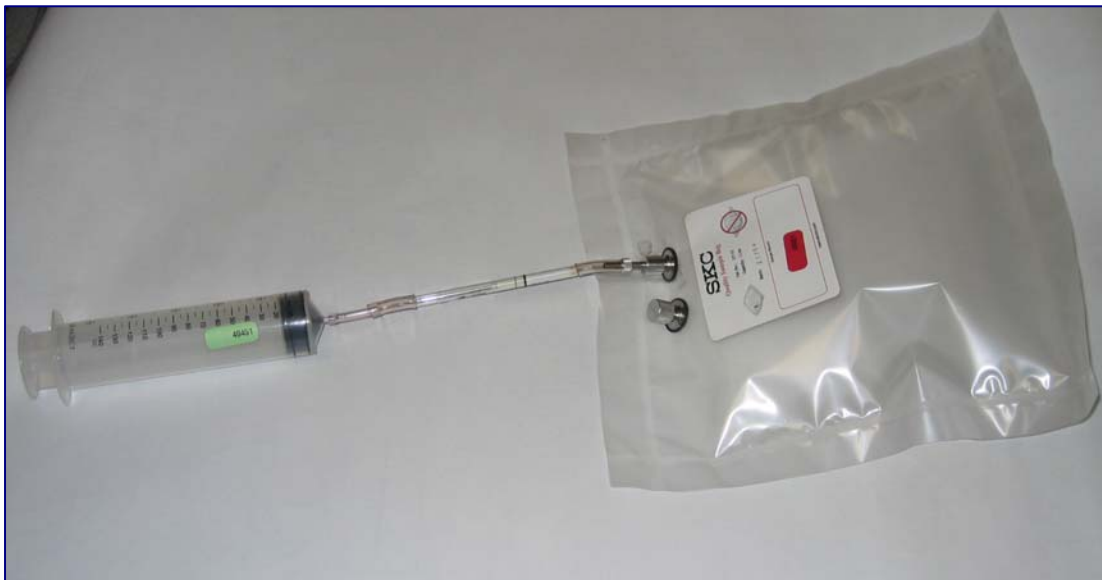
FIGURE 5-4 Diluted Sample Analysis with Dräger Tube
