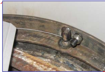
Strips of flat bar steel (40 mm width and 10 mm spacing) are welded to a flat ring.
