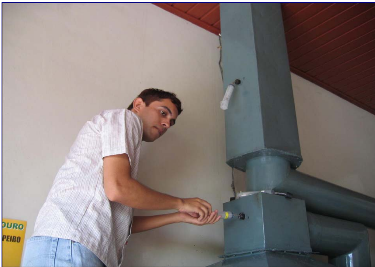
FIGURE 5-6 Sampling Train: Preparing to Draw a Sample
