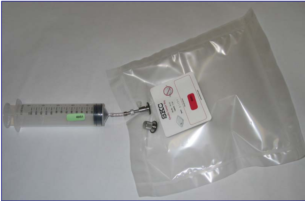
FIGURE 5-3 Sample in the Syringe Mixed with Clean Air in the Dilution Bag
