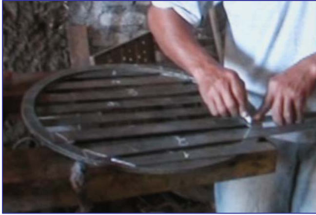
Strips of flat bar steel (40 mm width and 10 mm spacing) are welded to a flat ring.
