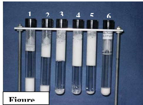
Figure 4. Flotation test of calcite powder treated with NA at different concentrations [Figure 4(a): TAN 0.4 ~ 0.5; Figure 4(b): 4 ~ 4.5]. Liquid phase: distilled water (pH~ 6). Solid treated with NA: (1) cyclohexanecarboxylic acid; (2) cyclohexanepropionic acid; (3) cyclohexanebutyric acid; (4) cyclohexanepentanonic acid; (5) trans-4-Pentylcyclohexane carboxylic acid; (6) without treatment.
