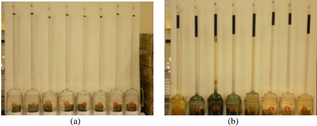
Figure 3. Photographs of 8 different Amott cell experiments taken a) at the start of the imbibition experiment and b) after about 3 weeks of elapsed time.
