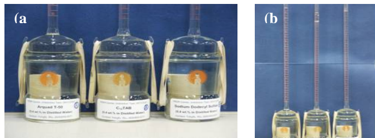
Figure 1(a), 1(b). Amott Cells used in imbibition oil recovery tests
