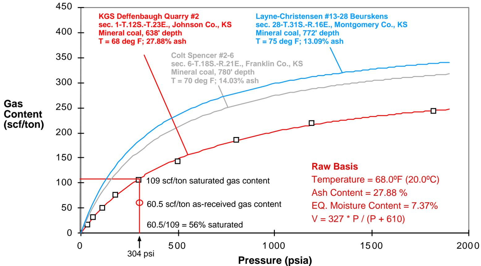
0.476 psi/ft X 638 ft depth = 304 psi reservoir pressure for Mineral coal
