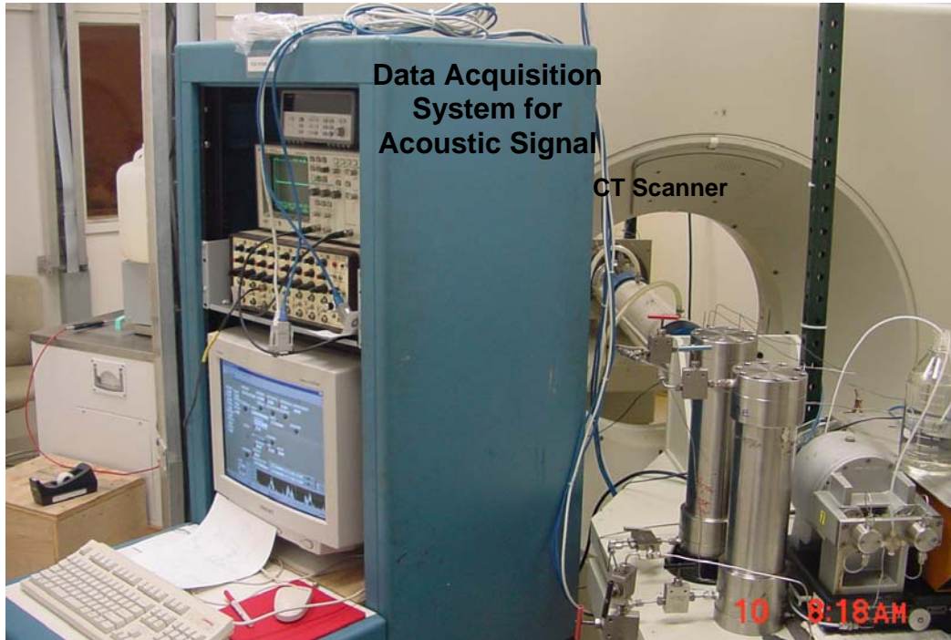
Figure 1.4. Experimental Setup (Front Side) for Hydrate Formation in Core
