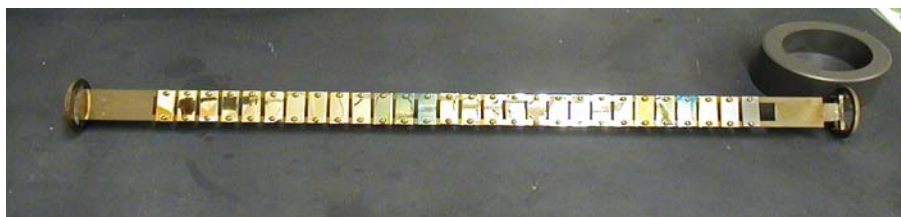
Figure 23. Sample geometry and design and the Inconel 625 corrosion sample holder, which can accommodate up to twenty eight samples.
