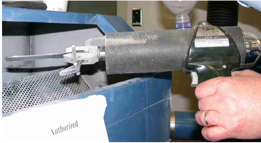
Figure 3. Cold spray facility at Westinghouse Corporation used for cold spraying zirconium-diboride coatings on various alloy substrates used in this study.
