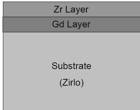
Figure 40. Schematic illustration of the multi-functional, multi-layered surface treatment to create a IFBA Gd-rich sub-surface layer and an outer corrosion resistant Zr layer.
