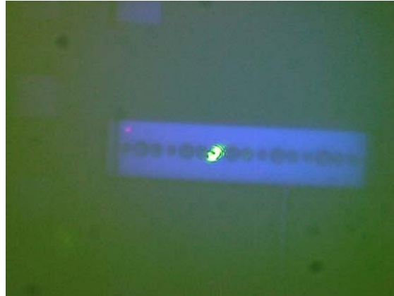
Figure 14 High power laser and LDV locations for second data set of optical excitation effect. Showing 10th hole with LDV in nominal position. (Root on right)
