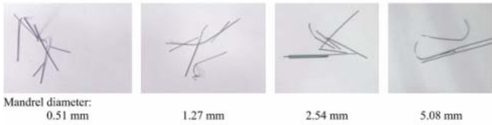
(a) Undoped Mo (0.254 mm diameter) after heating at 1300 °C.
