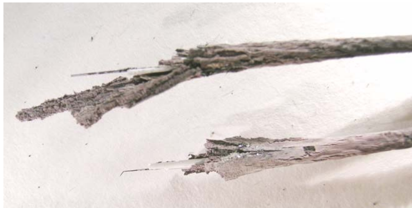
Figure 5-33. INL thermocouples (I15-11 and I15-12) after 3000 hours at 1500 °C.
