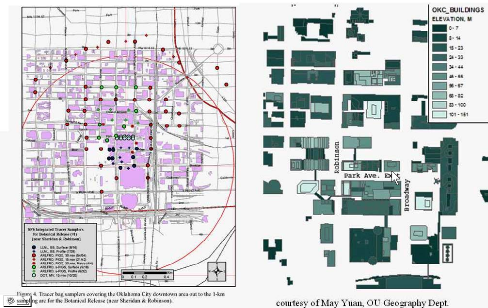
Figure 8: A map of sensor location placed in Oklahoma City during the Joint Urban 2003 full-scale dispersion experiment (Brown et al., 2004).
