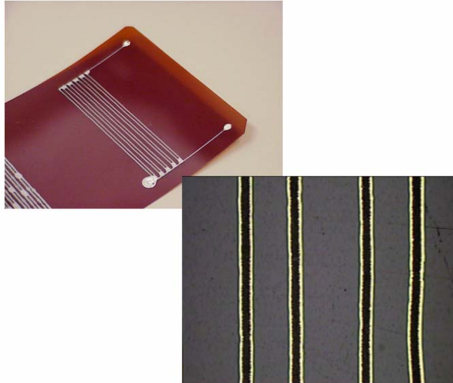
Figure 9: Printed silver lines on a Kapton Film(top). Close-up of needle printed silver lines (bottom).
