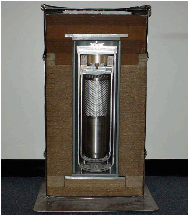
Figure 2. Representative installation of multi-filter-vented can and getter can assemblies, shown in cutaway.
