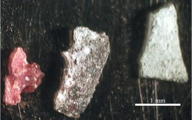
Figure 5 Particles of Slag #2 (1000-1500 µm) as received (left), after two hours of reaction (center), and after 96 hours of reaction (right)
