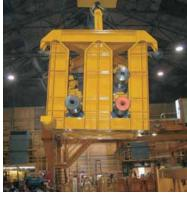
6 Moving rolls in cassettes reduces handling time by up to 85%
