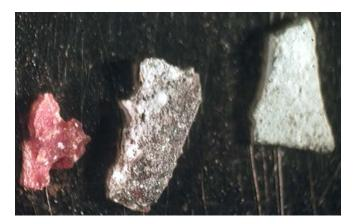
Figure 5 Particles of Slag #2 (1000-1500  $\mu$ m) before the reaction with CO<sub>2</sub>/water (left), after two hours of reaction (center), and after 96 hours of reaction (right)
