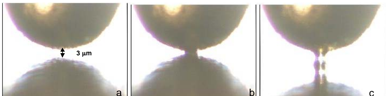
Figure 3. Movie frames showing out of contact cavitation at a distance of \sim 3 micron a) one frame prior to b, b) clip showing cavitation, and c) extended vapor cavity visible during withdrawal. Bottom semicircular shape is a reflection of the spherical SH tip from the underlying flat SH surface.
