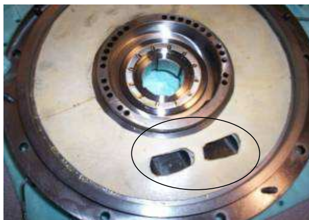
Figure 42: This figure shows the insulator material after being modified to provide the oil passage holes.
