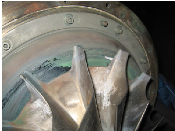
Figure 46: Turbine and Turbine Backplate Damage
