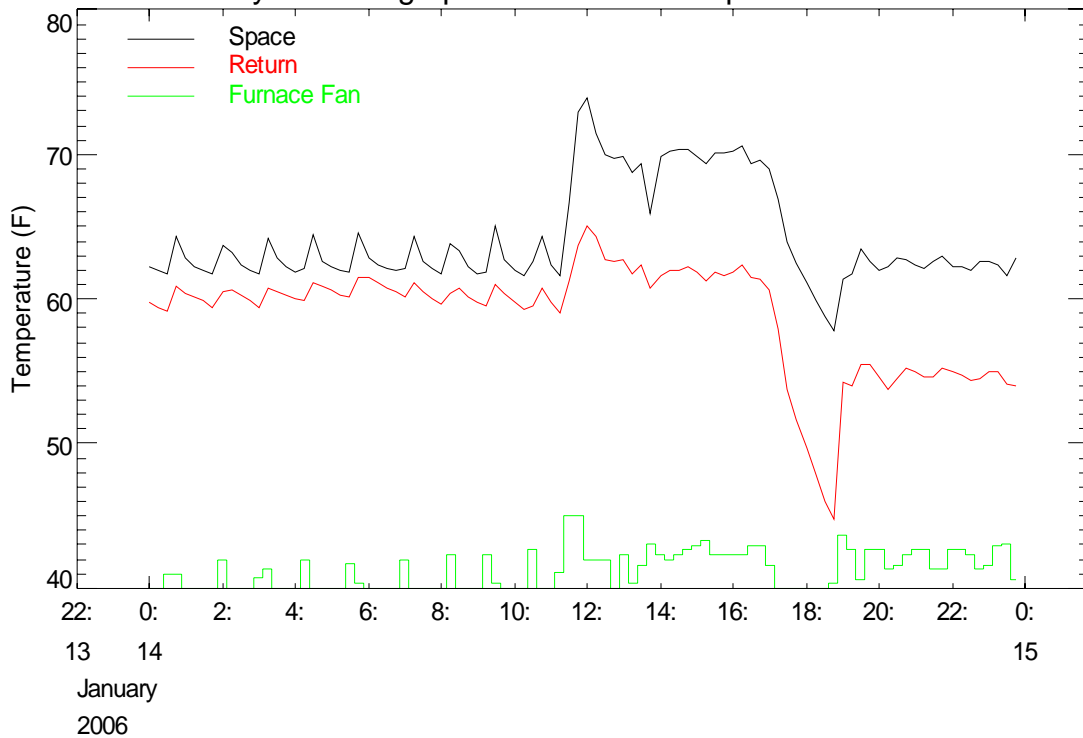
Figure A2-39. Space and Return Conditions For Base Building Typical Day with Setback
