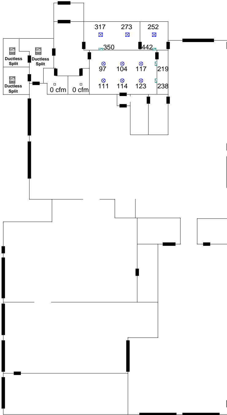
Figure A11-16. Supply and Return Airflow Measurements (cfm)
