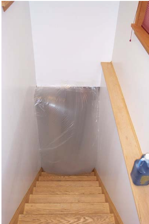
Figure A25-4. Entrance to Basement Sealed and Bathroom Exhaust Covered (Test 2)
