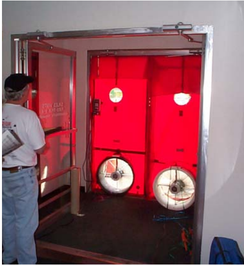
Figure A4-10. Two Blower Doors Setup for Depressurization (Main Entrance)
