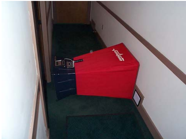
Figure 2-5. Air Flow Measurements with Compensated Flow Hood
