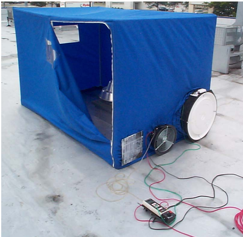
Figure A24-9. Exhaust Fan Capture Tent (Typical Installation)
