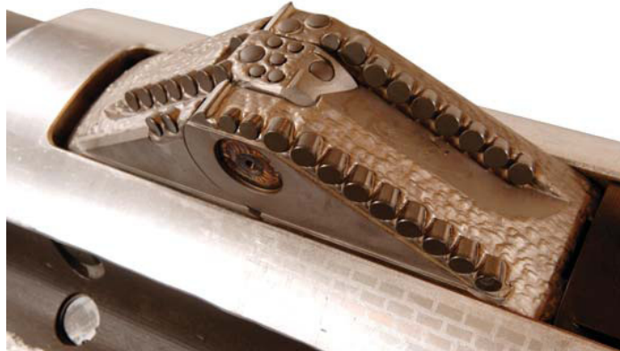
C-5 Halliburton under-reamer
