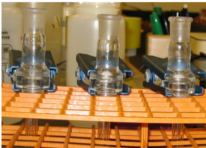
Figure 12. Photograph of glass filter holders used to test biocidal activity on ceragenin-treated RO membranes.
