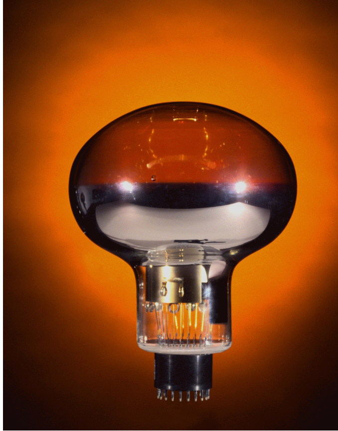
FIGURE 2.5. A picture of a 8-inch PMT used in the MiniBooNE experiment
