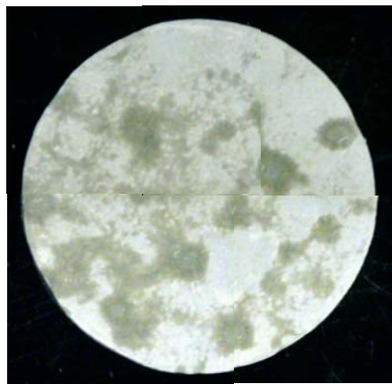
Figure 18. A composite optical micrograph of a 0.25 mol% Bi 2 O 3 sample after 16 hr at 725°C.
