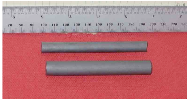
Fig. 18 Sintered SFC2 tube prepared by cold isostatic pressing of SFC2 powder.
