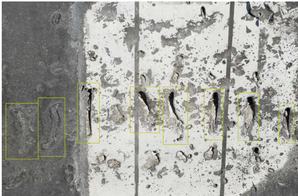
Figure 16: Witness plate from the test article. Notice the fragment strip indentations highlighted in yellow.
