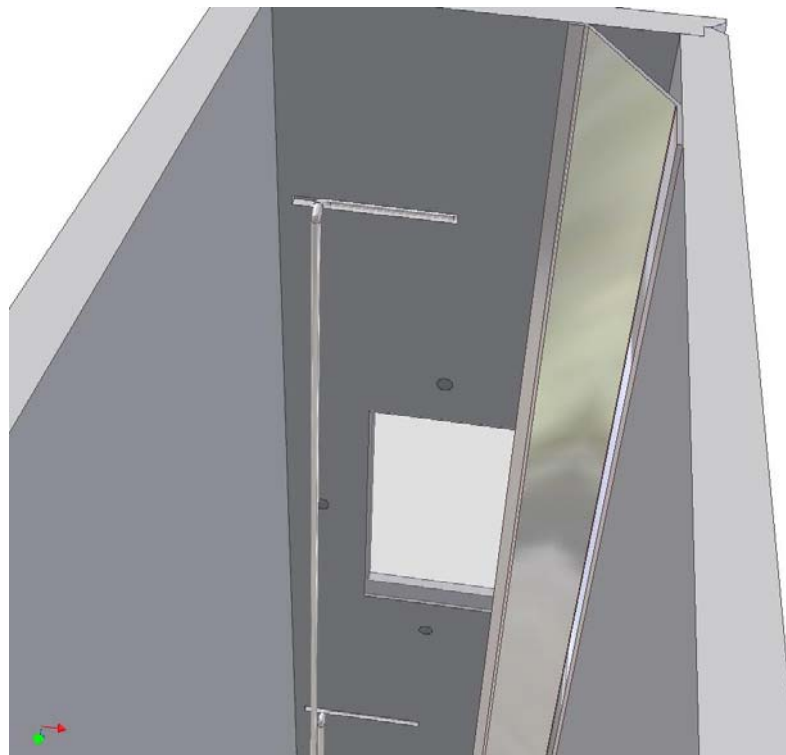
Figure 5.10. Tube Interior View Showing Thermocouple and Viewport Installation Details.
