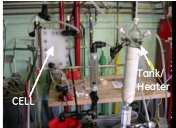
Figure 10: Bench-scale single cell test device
