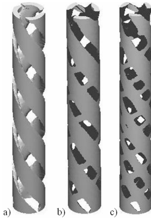
Figure 25. Results for f_r/f_t=1 , \nu_f=0.12 and: a) 5452 Finite Elements, b) 19584 Finite Elements, and c) 49632 Finite Elements.
