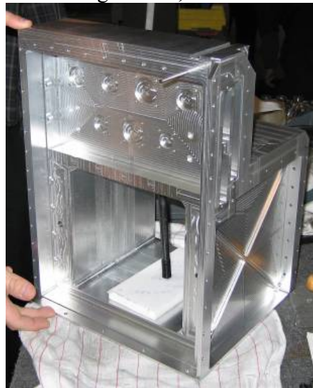
Figure 1. Aerospace Electrical Housing Showing Lightweighted Rib-On-Plate Structure.
