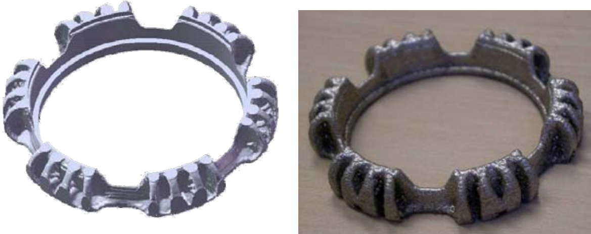
Figure 51. ATO Optimized 3D Lens Housing (left) and LENS Manufactured Housing (right).
