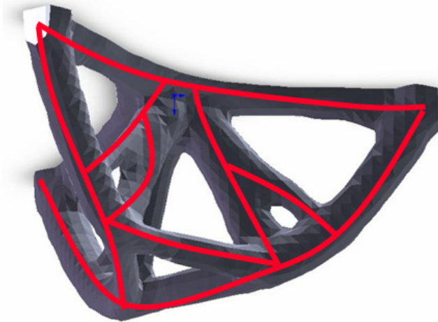
Figure 44. This optimized structure has medial axis splines that were sketched onto the surface of the part by a user.
