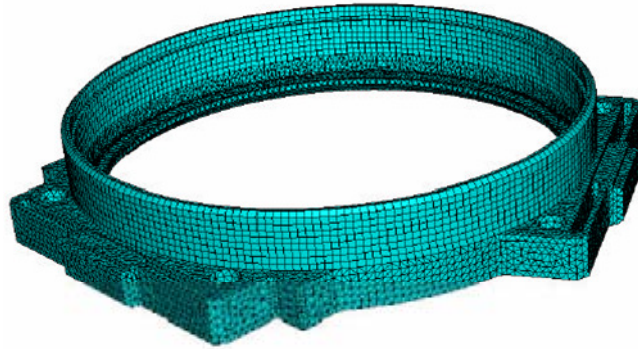
Figure 48. Finite Element Mesh of Lens Housing.
