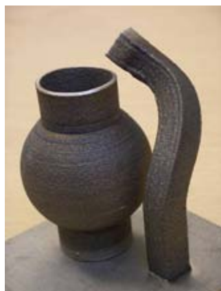
Figure 46. Curved 3D Parts Built From 316 Stainless Steel Using the LENS Process.
