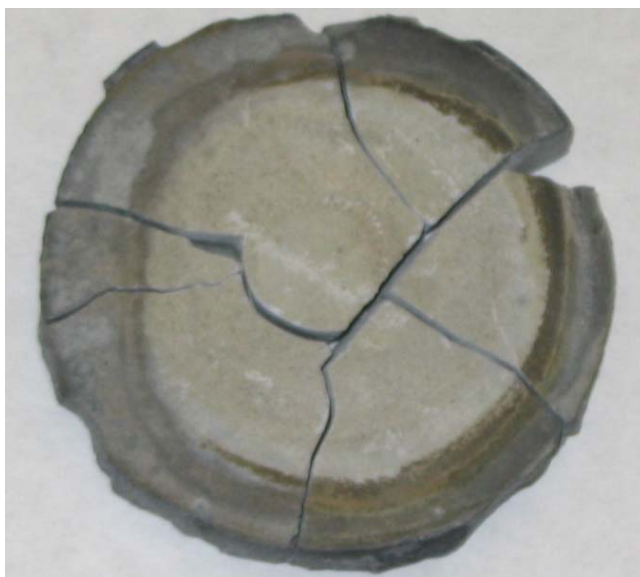
Figure 8. Picture of the shattered SnO 2 /SnF 2 target used for sputter deposition of the F-SnO 2 thin films.
