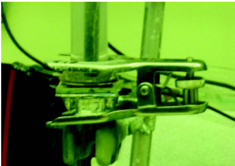
Figure 9. O-ring seal for electrolysis testing of tin oxide and ruthenium oxide films.
