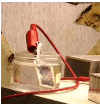
Figure 26. Gas generation of the triple junction solar cell coated with Flexbond-ATO (30 v %) composite film under a halogen light.
