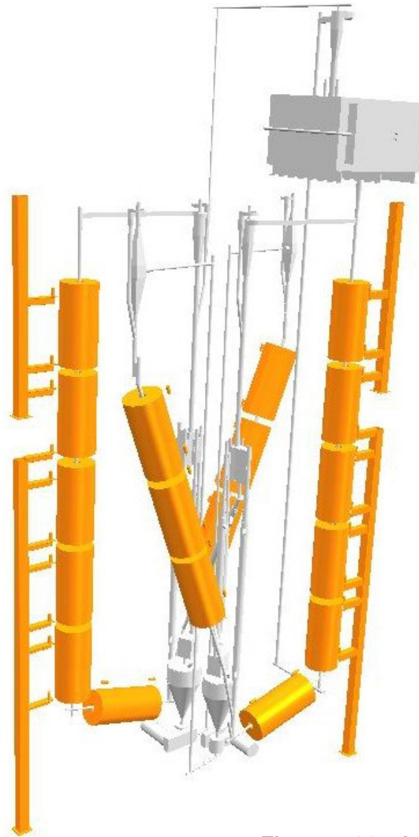
Figure 5-23 – Location of Electrical Heaters and Supports
