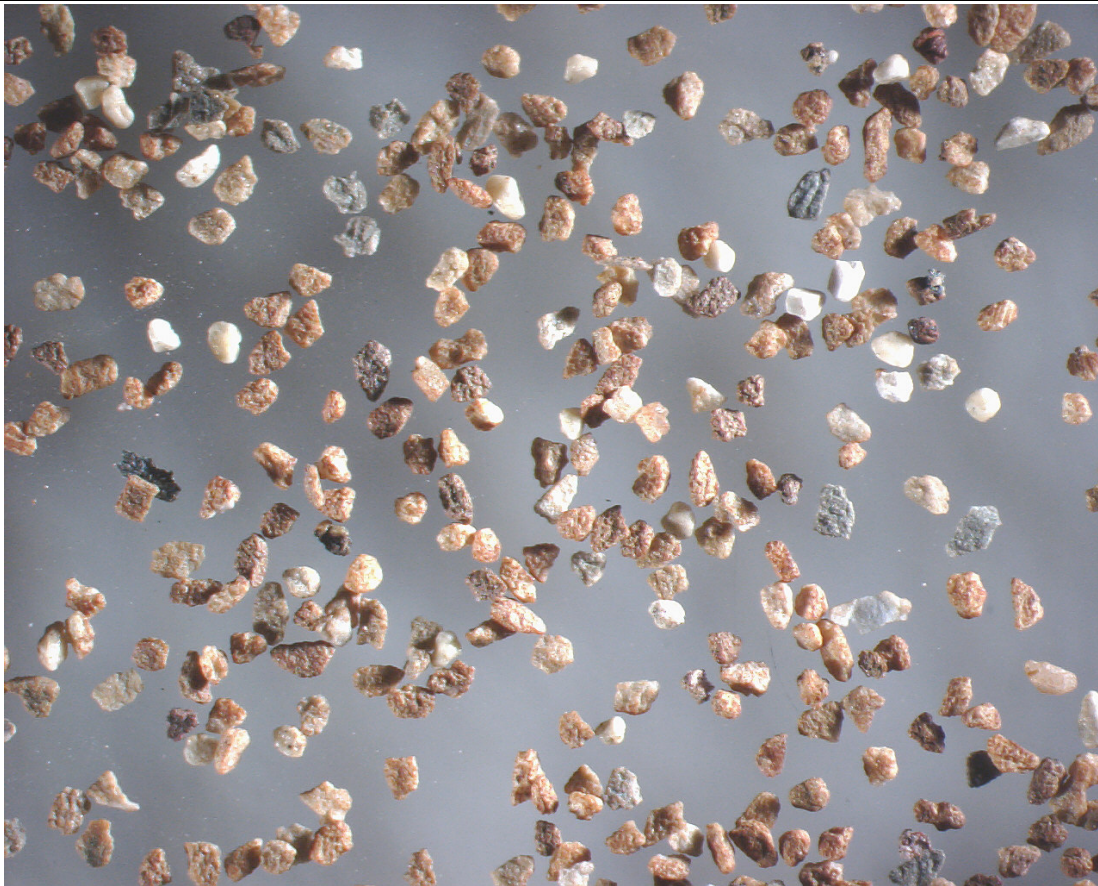
Figure 8-23 - Particle shapes for 120mesh screen sample
