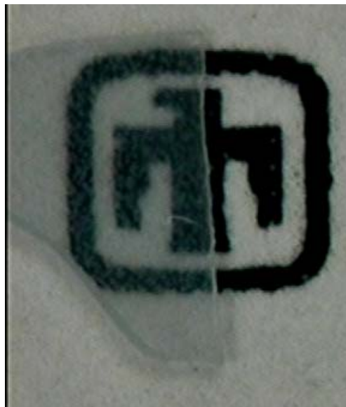
Figure 15. Photograph of YAG sample that was vacuum sintered at 1650°C for 5 hr.
