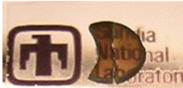
Figure 29. A hot-pressed sample of GSGG-13.
