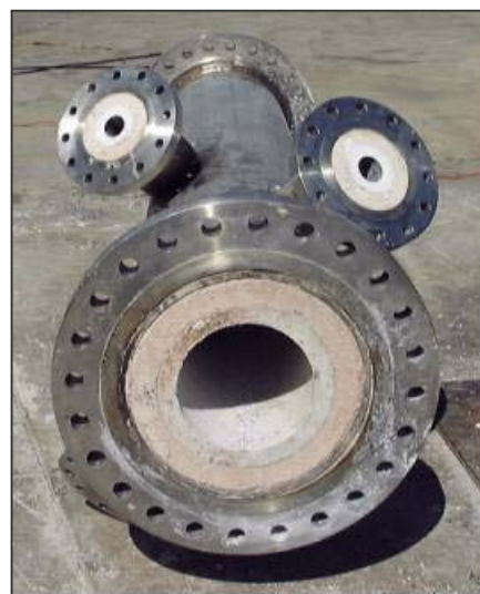
Figure 2-9. Photo of R1 shell with two cast refractory layers.
