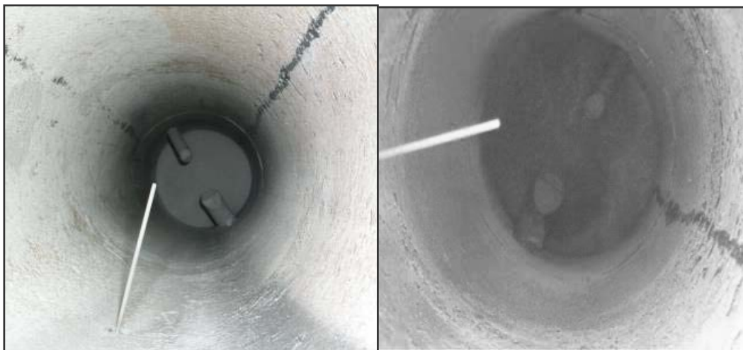
Figure 3-16. Photo showing inside of pilot-scale R2 fluidized bed, with two solids transfer inlet ports (near bottom) and one thermocouple (near top) with a static bed (left photo) and during filming of a solids transfer test (right photo).
