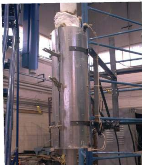
Figure 2-2. Furnace surrounding outer shell of lab-scale reactor.
