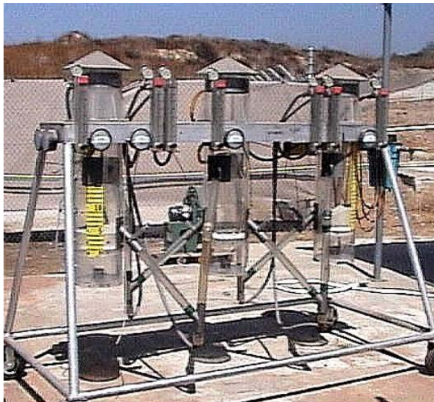
Figure 2-5. Cold flow model of solids transfer.
