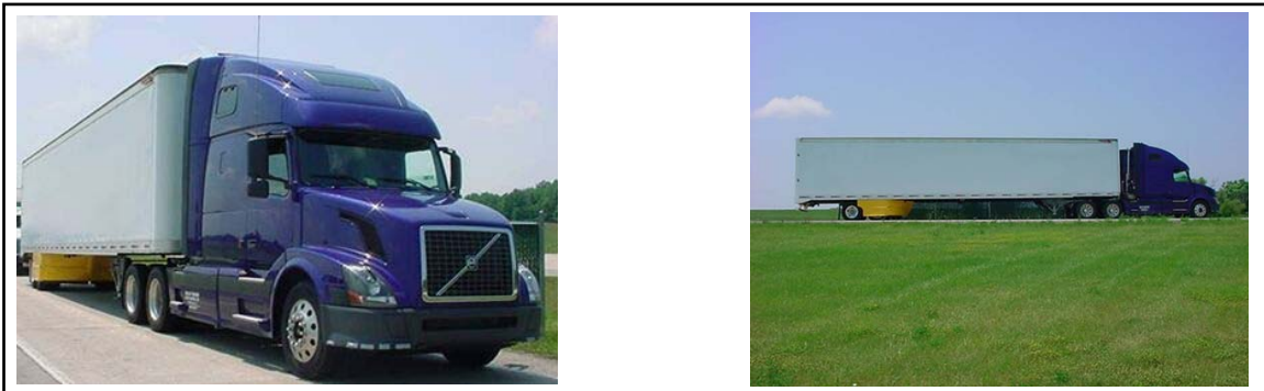
Figure 6-25. Test 2 VN 670 – Total Combination of Tractor and Trailer Mounted Devices
