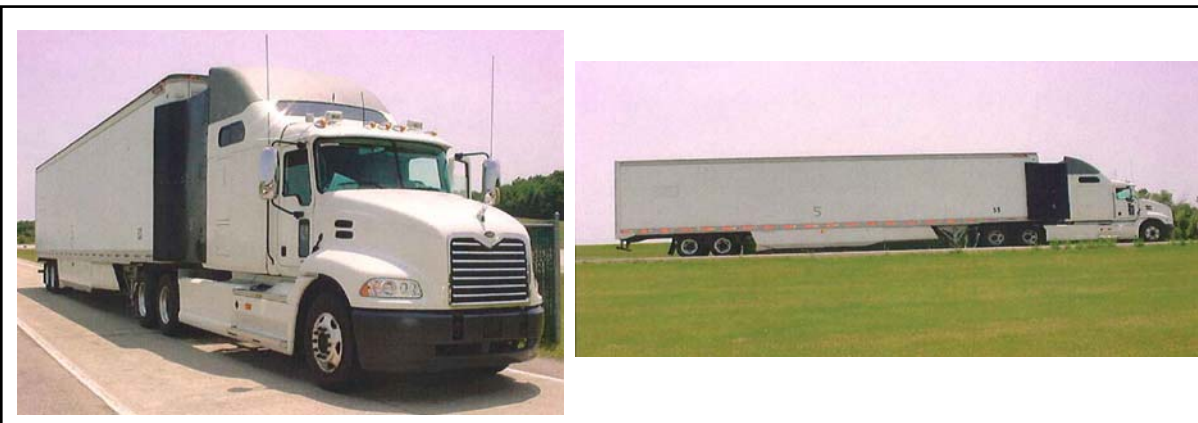
Figure 5-19. Test 4 – Side Enclosure and Side Skirts
