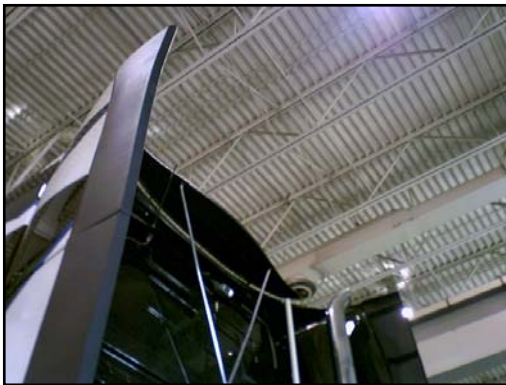
Figure 6-18. Side Deflector Extensions and Adjustable Roof Extender
