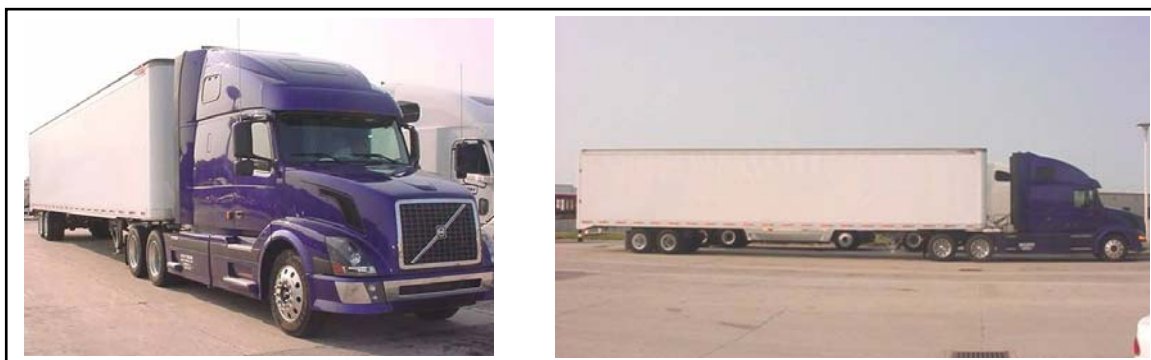
Figure 6-28. Test 5 VN 670 – Gap Devices and Deck Closure
