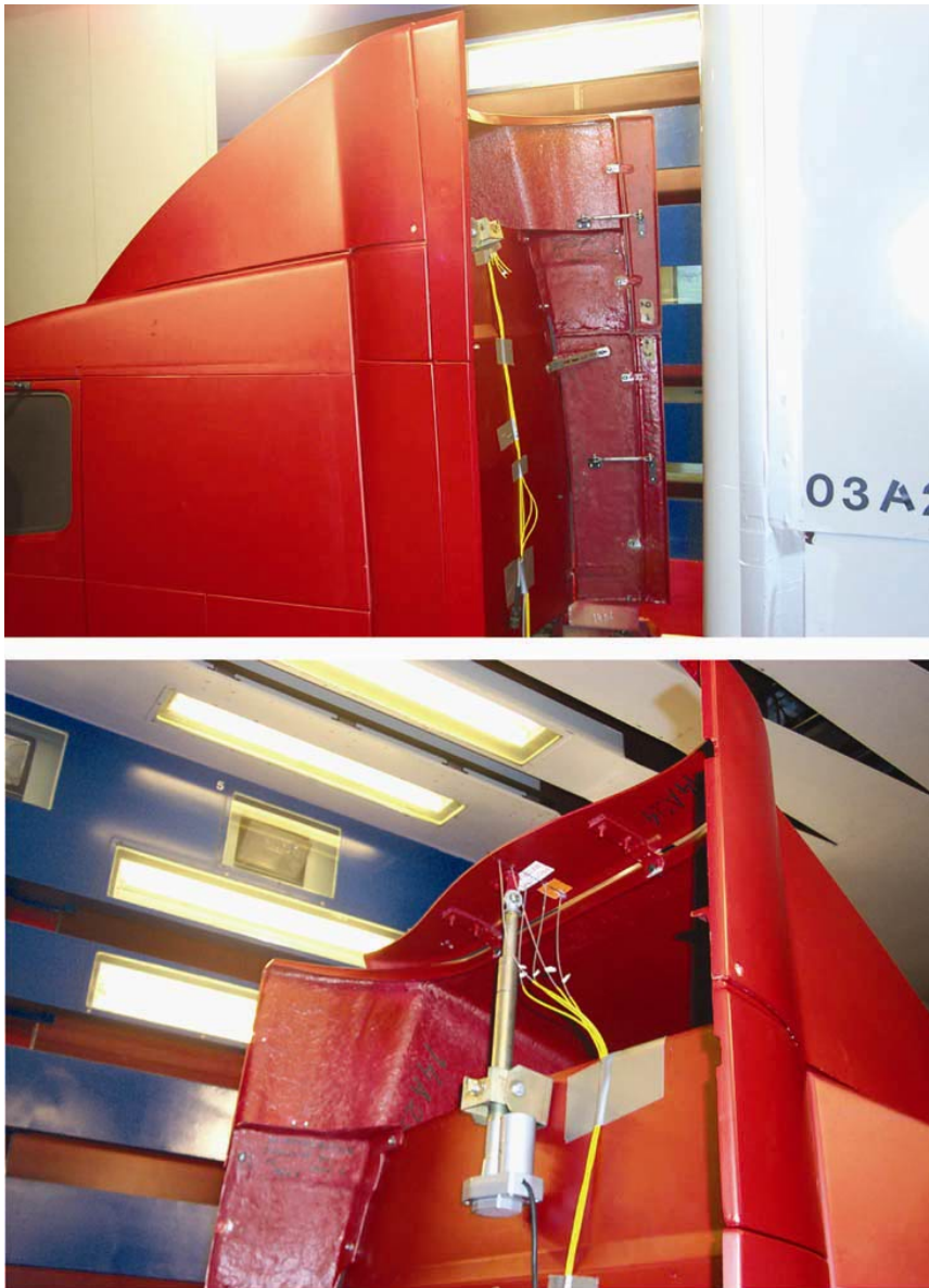
Figure 6-7. Sample Trailer Gap Flow Controls: Side Deflector Extensions (Top) and Roof Extenders (Bottom)
