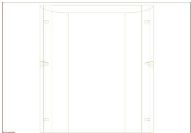
Figure 4-26. 15 degree, Flat Design, Front View (Trailer Forebody Device, CAD Image)
