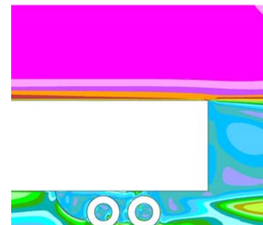
Figure 6-15. CFD Analysis of Proposed Trailer Bogie Deflector
