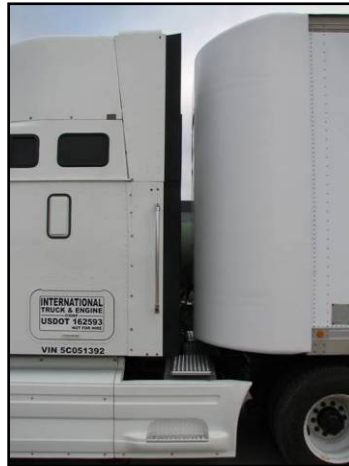
Figure 4-27. 15 degree, Flat Design, Installed on Trailer (Trailer Forebody Device, Prototype Part)
