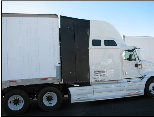
Figure 4-29. Variable Length Side Extenders -- Deployed
