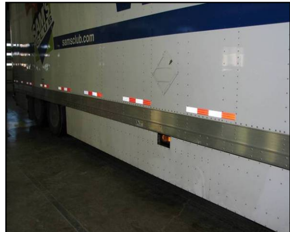
Figure 4-23. Trailer Skirts Deployed on Wal-Mart Experimental Aerodynamic Trailer
