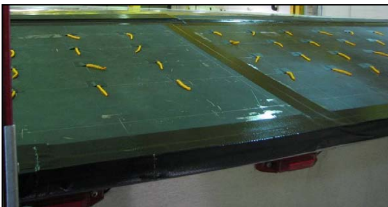
Figure 4-31. Yarn tufts on smooth panels covering tapered roof section of trailer
