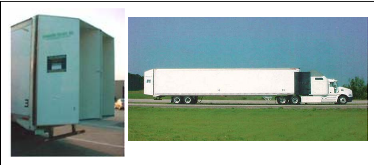
Figure 5-18. Test 3 – Side Enclosure and 4 Foot Boat Tail
