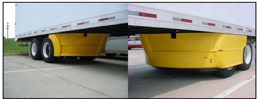
Figure 6-19. Two Different Trailer Bogie Concepts Studied in Phase II
