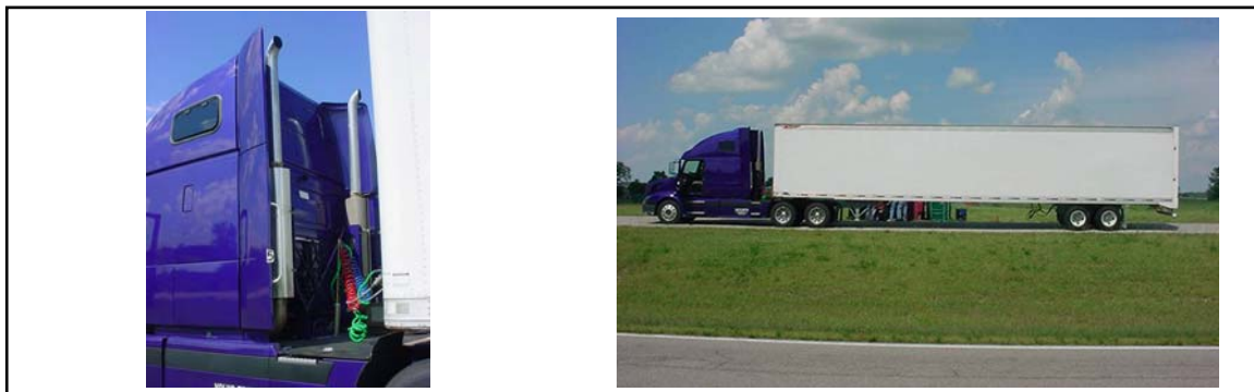
Figure 6-27. Test 4 VN 670 – Gap Devices and Deck Closure
