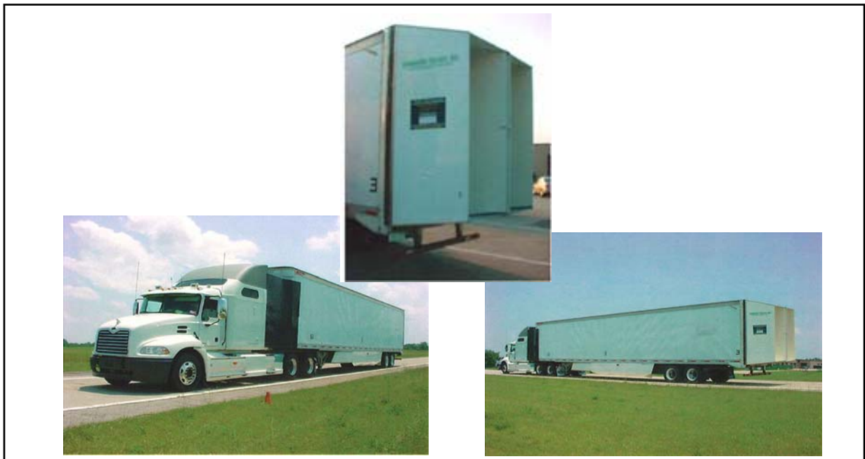
Figure 5-16. Test 1 – Side Enclosure, 4 Foot Boat Tail, and Side Skirts
