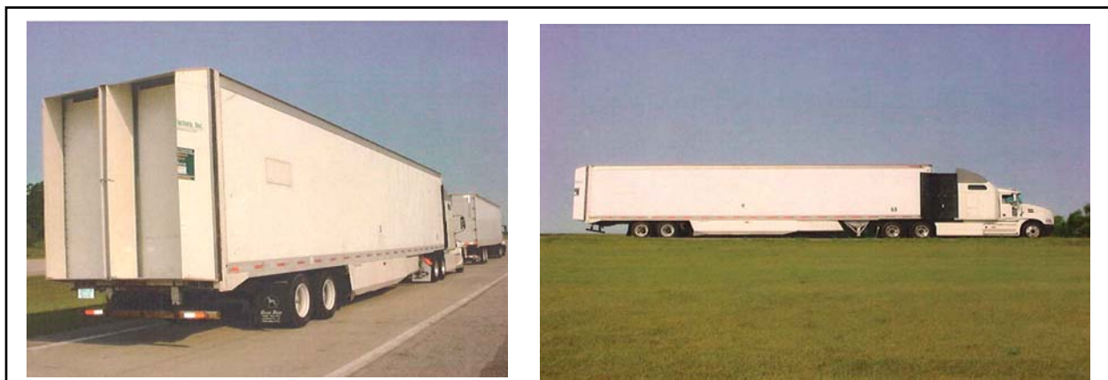
Figure 5-17. Test 2 – Side Enclosure, 2 Foot Boat Tail, and Side Skirts
