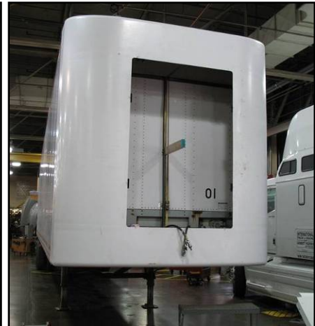
Figure 4-28. 5 degree, Flat Design, Installed on Trailer (Trailer Forebody Device, Prototype Part) Note: Access panel removed in photo
