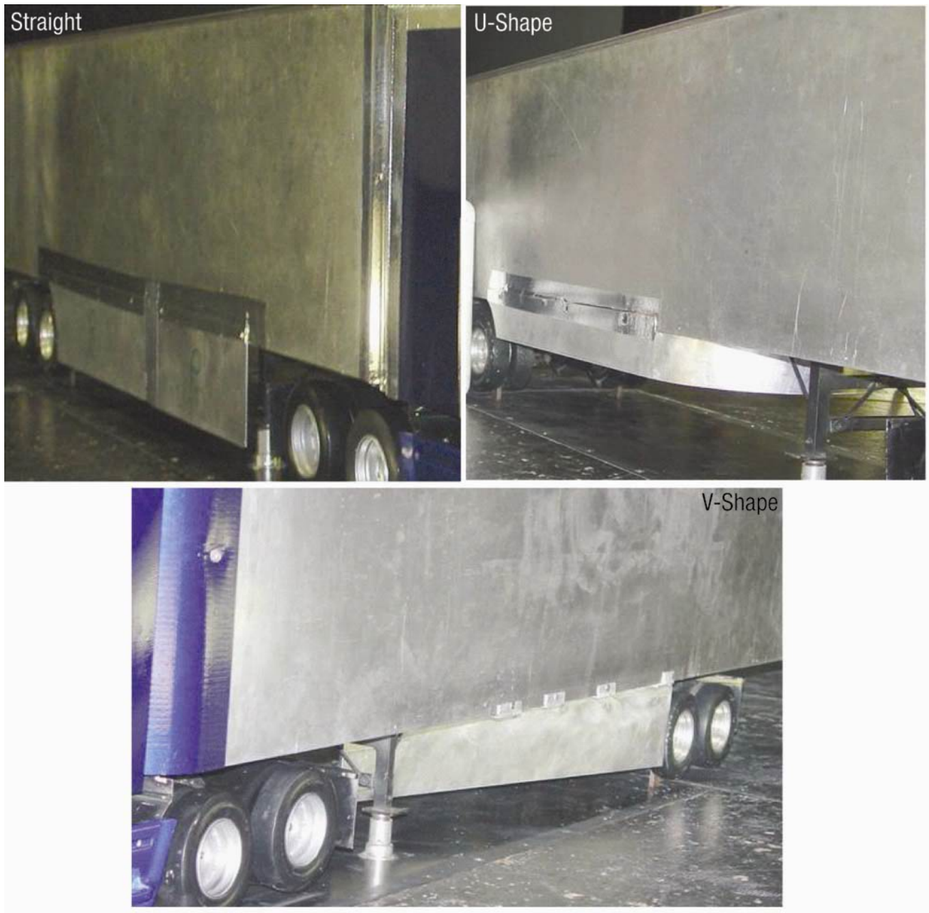
Figure 4-12. Various Side Skirt Shapes Tested in Wind Tunnel
