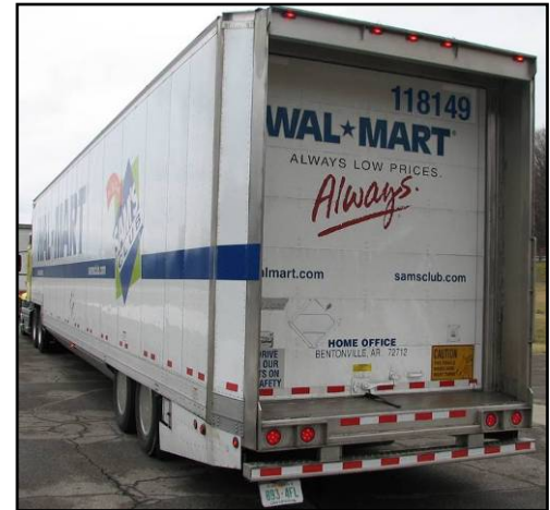
Figure 4-24. Tapered Aft Section of Trailer (Wal-Mart Experimental Aerodynamic Trailer)
