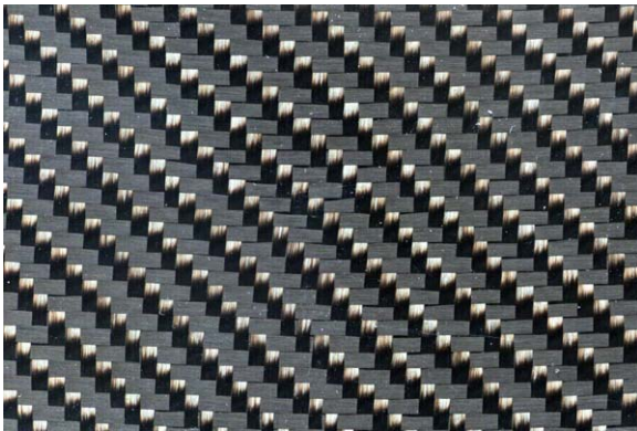
Figure 2. Typical CF woven cloth
