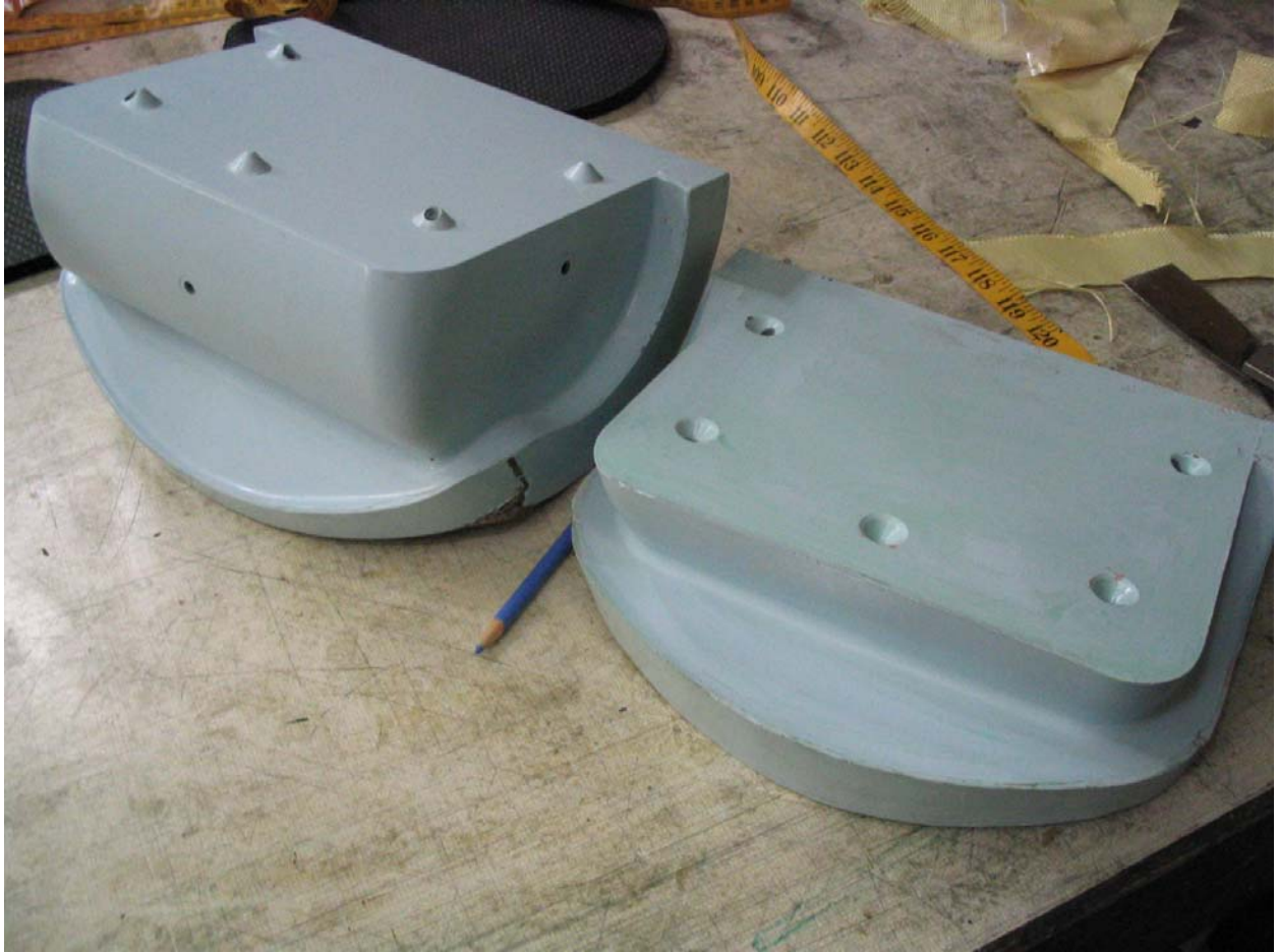
Front and back half female molds.
