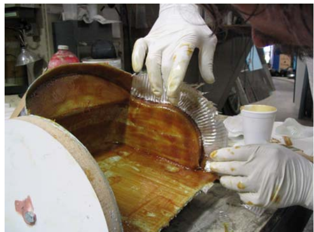
Figure 24. Creating the female mold in fiberglass weave
