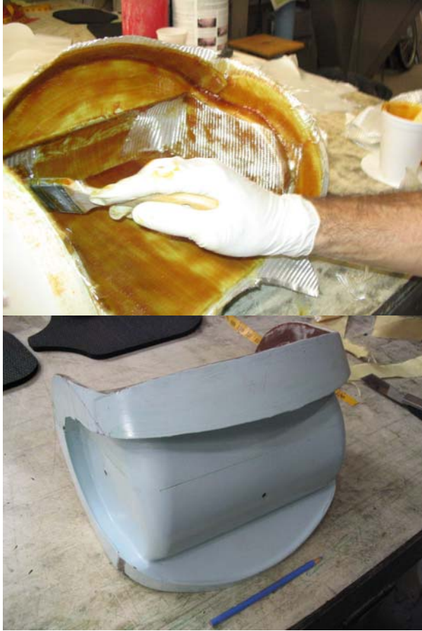
Figure 25. Finished Lower Female Mold with RP male part fitted
