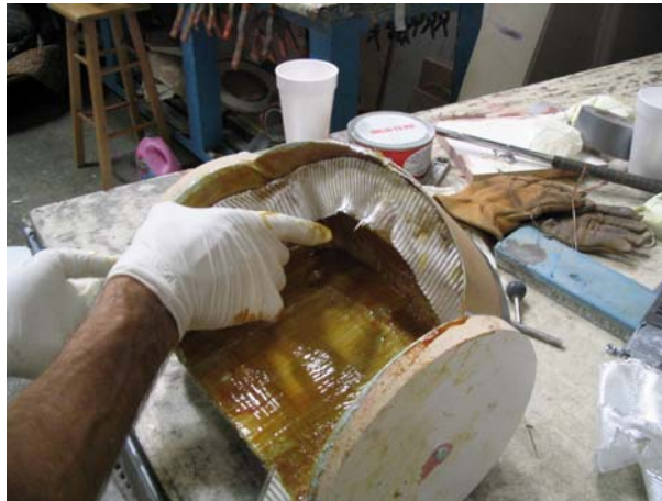
Figure 24. Creating the female mold in fiberglass weave
