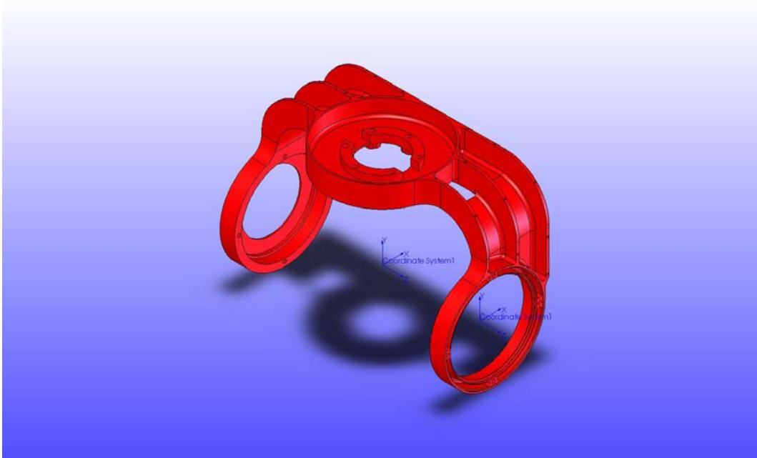
Figure 1. Aluminum MiniSAR outer gimbal arm
