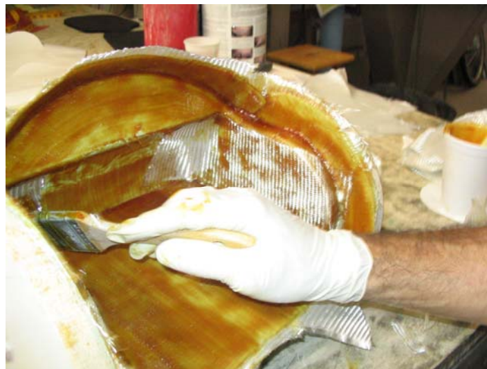
“Wetting out” the fiberglass fabric with more resin.
