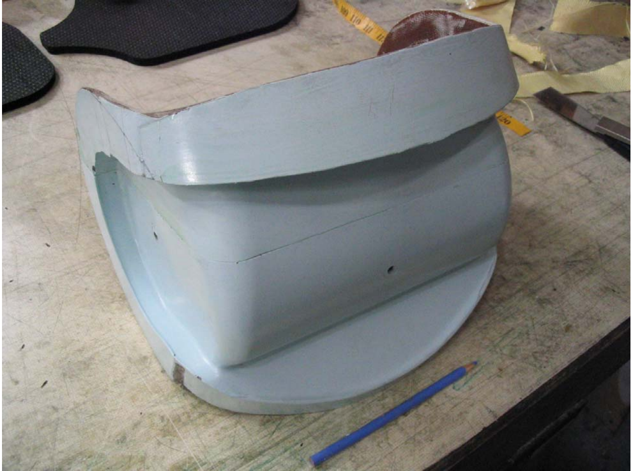
Assembled front and back halves ready for final male part layup.
