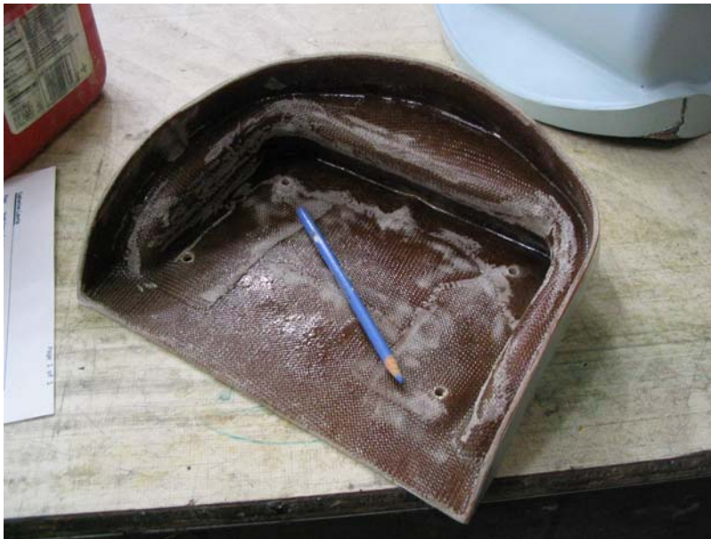
Female mold separated from RP part.
