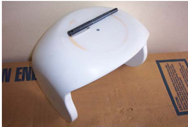
Figure 23. RP part ready to be used for female mold fabrication
