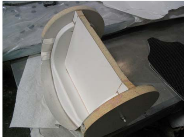
Using the Rapid Prototype (RP) part to fashion the female molds.
