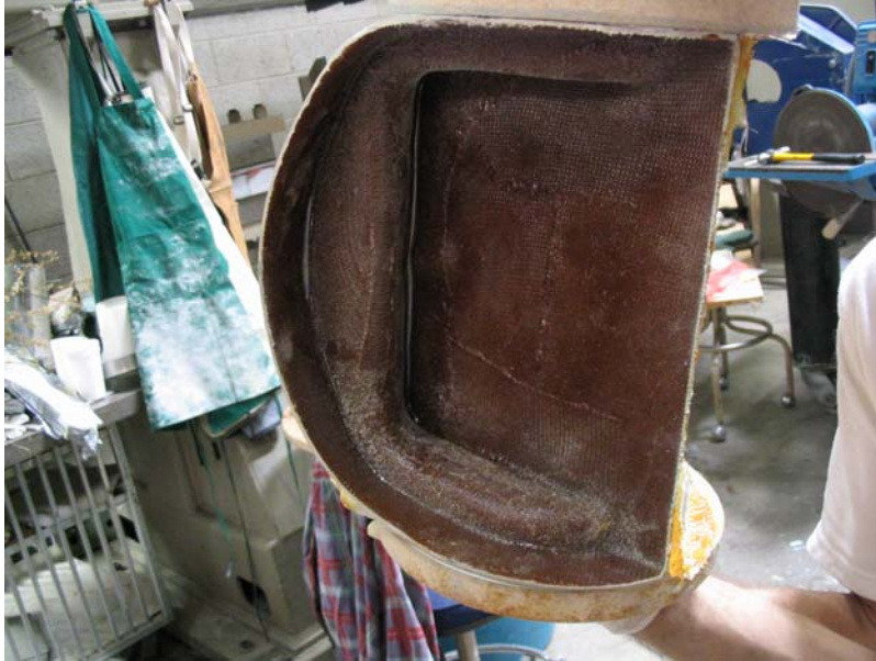
Cured female fiberglass mold on male RP part.
