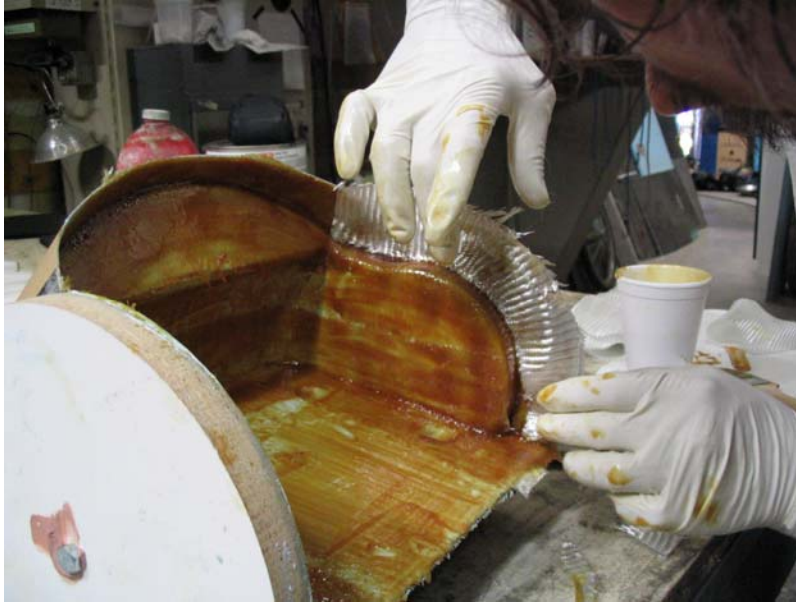
Applying fiberglass weave directly to wet resin, on top of male RP part.
