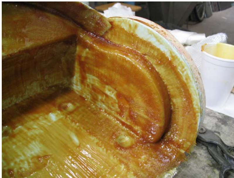
Wet lay-up of epoxy resin applied to male part.
