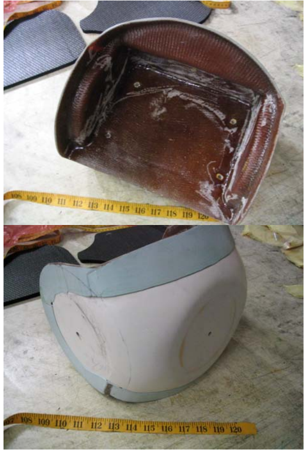
Figure 25. Finished Lower Female Mold with RP male part fitted
