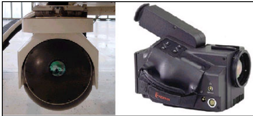
Figure 12. Helicopter-Mounted (L3 Corp.) and Hand-Held (Agema) Thermal Imagers
