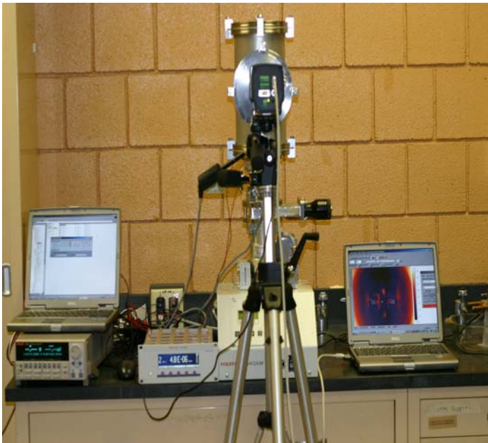
Photos of custom vacuum test setup with IR camera
