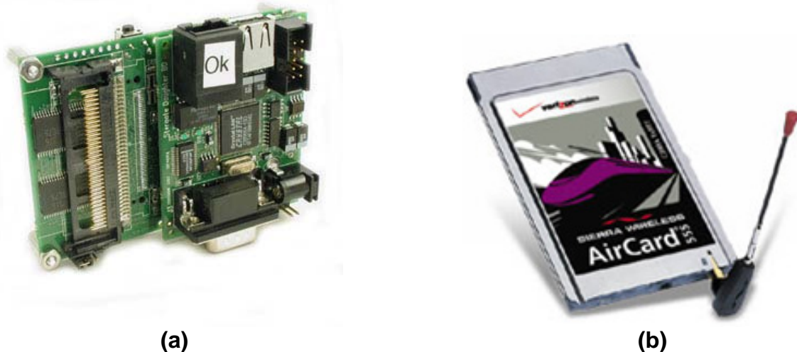
Figure 3-14 (a) Stargate system; (b) Cell phone modem that plugs into Stargate.
