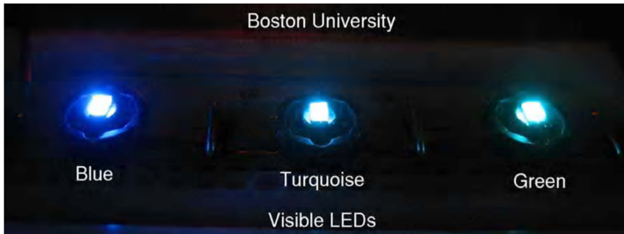
Figure 51: Semi-packaged LEDs of different colors grown by MBE on smooth HVPE GaN templates. All three devices were injected with the same current
