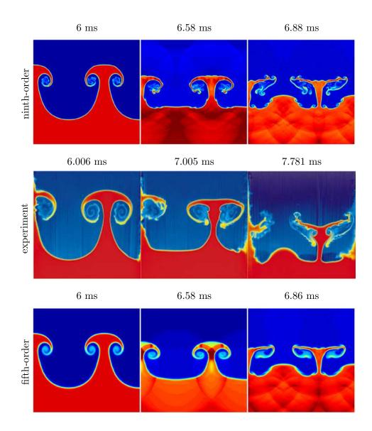
FIG. 2: (Color). Further comparison of corrected PLIF images from the experiment of Collins and Jacobs<sup>15</sup> and the density from the fifth- and ninth-order WENO simulations at selected times just before and after reshock of the evolving interface. The experimental images are taken from Fig. 6 of Collins and Jacobs (reprinted with the permission of Cambridge University Press).
