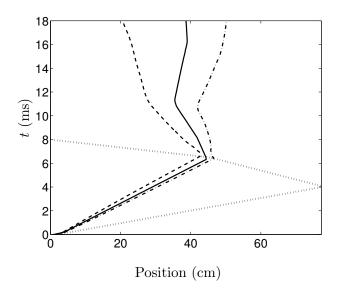
FIG. 5: The *x*-*t* diagram showing the position of the interface  $\ell_{int}(t)$  (solid line), shock (dotted line), and bubble and spike tip locations  $\ell_b(t)$  and  $\ell_s(t)$  (dash-dot and dashed lines, respectively) from the ninth-order simulation. The horizontal distance between the spike and bubble tip location is the mixing layer width h(t).
