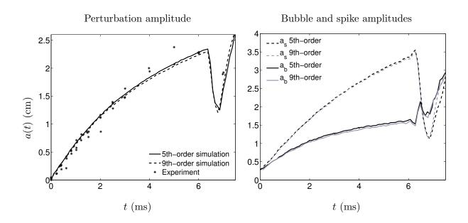
FIG. 6: Comparison of the amplitude obtained from the fifth- and ninth-order WENO simulation to the experimental data points from Collins and Jacobs<sup>15</sup> (left). The bubble and spike amplitudes from the simulations,  $a_b(t)$  and  $a_s(t)$ , respectively, are also shown (right).
