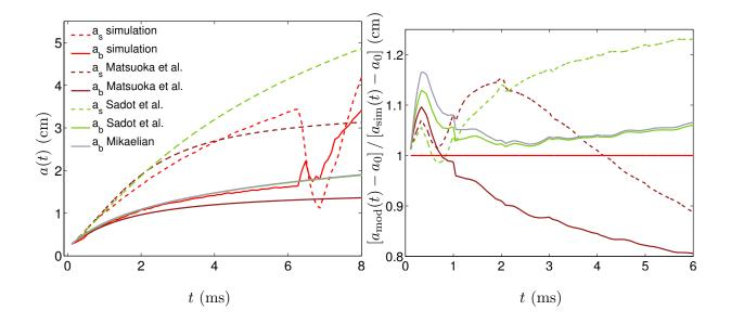
FIG. 11: (Color). Comparison of the bubble and spike amplitudes,  $a_b(t)$  and  $a_s(t)$ , from the ninth-order WENO simulation with the predictions of the Matsuoka *et al.* (Padé) and Sadot *et al.* models, and with the Mikaelian model in the case of the bubble amplitude (left). Also shown are the ratios of the model predictions to the simulation bubble and spike amplitudes (with the initial perturbation amplitude subtracted out) (right).
