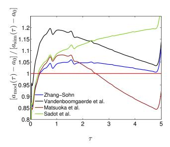
FIG. 10: (Color). The predictions of the Zhang-Sohn (Padé), Vandenboomgaerde *et al.* (Padé), Matsuoka *et al.* (Padé) and Sadot *et al.* models (with the initial perturbation amplitude subtracted out) divided by the corresponding ninth-order WENO simulation amplitude.
