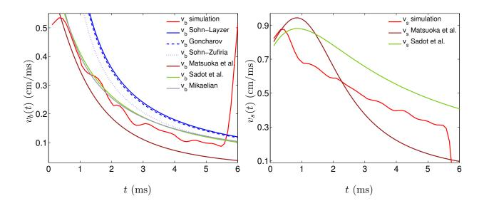
FIG. 12: (Color). The bubble velocity,  $v_b(t)$ , from the ninth-order WENO simulation with the asymptotic velocities predicted by the Goncharov, Sohn-Layzer and Sohn-Zufiria models and the velocities predicted by the Matsuoka *et al.*, Sadot *et al.* and Mikaelian models (left). Also shown is the spike velocity,  $v_s(t)$ , and the velocities predicted by the Matsuoka *et al.* and Sadot *et al.* and Sadot *et al.* models (right).
