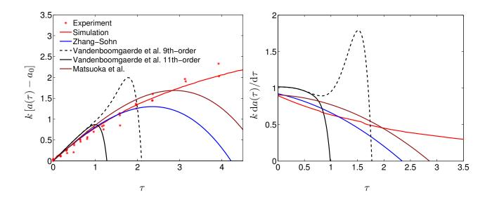
FIG. 8: (Color). The normalized amplitude  $k[a(\tau) - a_0]$  versus  $\tau$  from the ninth-order WENO simulation and the experimental data points, together with the predictions of the Zhang-Sohn, Vandenboomgaerde *et al.* and Matsuoka *et al.* perturbation series models (left). The normalized growth rates  $k da(\tau)/d\tau$  versus  $\tau$  from the ninth-order simulation, together with the corresponding growth rates from the perturbation series models, are also shown (right).
